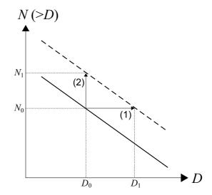
Fig. 5. Schematic illustration of the change of crater SFD due to apparent change of crater size. D is crater diameter, and N(>D) is the cumulative number of craters whose diameter is greater than D. Adopted and modified from Ishizaki & Furumoto (1997).
