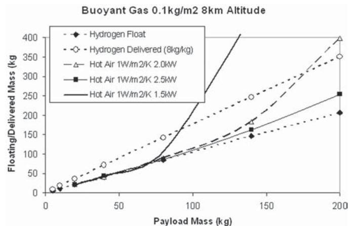
**Fig. 7** Mass Tradeoff between Hot air and buoyant gas for tropospheric balloons. Until the hot air performance threshold is reached (~200 kg for 2 kW and 1 W/m<sup>2</sup>/K) the hot air balloon has a comparable float mass but much lower delivered mass than a hydrogen balloon.
