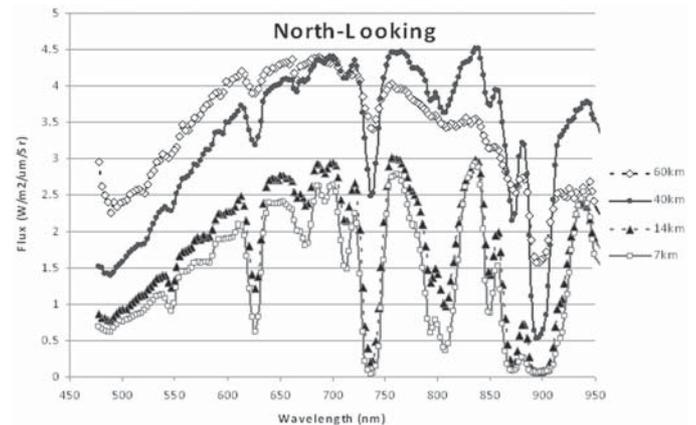
**Fig. 11** Upward-looking visible and near-IR fluxes recorded by the Huygens probe DISR instrument. (PDS Dataset ID HP-SSA-DISR-2/3-EDR/RDR-V1.0 ULVS\_DDP.TAB). Flux is relatively insensitive to altitude in the lower troposphere, but is rather higher at 40-60 km.
