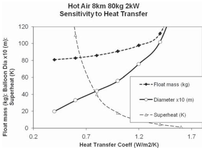
Fig. 8 Hot air balloon parameters are acutely sensitive to assumed heat transfer coefficient. For nominal performance ( $\sim 1 \text{ W/m}^2/\text{K}$ ) the required balloon diameter is  $\sim 8\text{m}$  with a superheat of  $\sim 20 \text{ K}$ .
