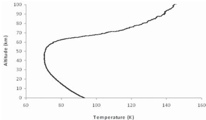
Fig. 3 Titan atmosphere temperature profile as measured by the Huygens Atmospheric Structure Instrument.
