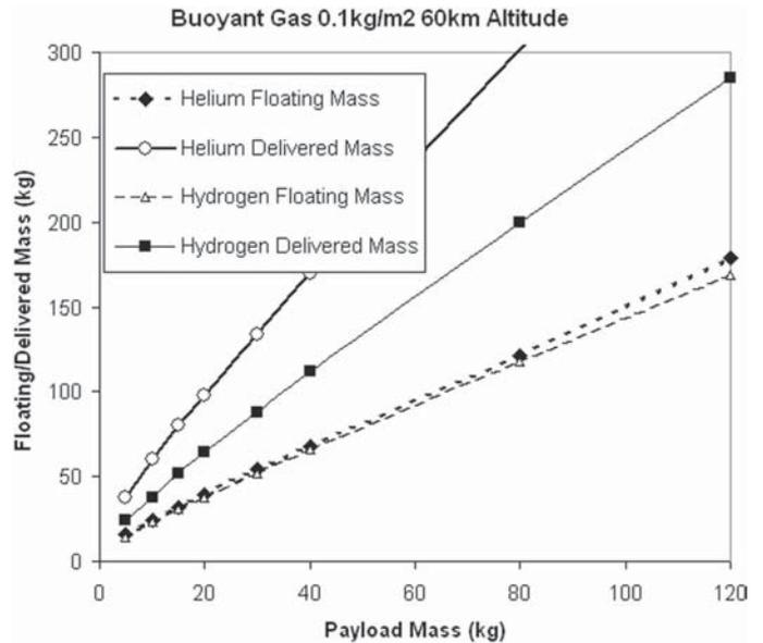
**Fig. 6** Stratospheric buoyant gas balloons have envelope masses that are small relative to the payload. Delivered mass (float mass plus gas and tankage) is sensitive to choice of fill gas, with hydrogen offering superior performance assuming tankage fraction is the same for both (8 kg/kg).
