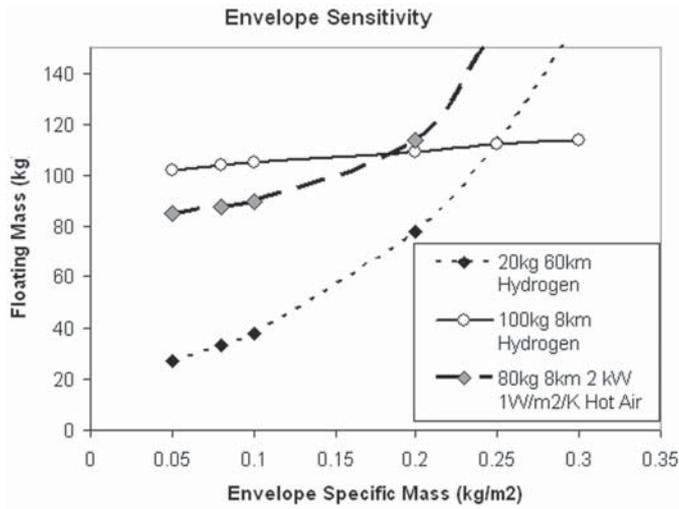
**Fig. 5** For a tropospheric hydrogen balloon, and a tropospheric hot air balloon well within performance limits, float mass is relatively insensitive to envelope material density. For hot air near its limit, and for a stratospheric hydrogen balloon, envelope specific mass becomes a significant factor.
