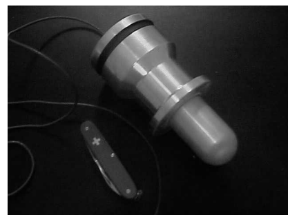
Fig. 10. Assembled Test article. The black recessed band on the sabot indicates where a graphite shear pin holds the projectile inside the gun barrel. The cable is coiled inside the rear part of the sabot.
