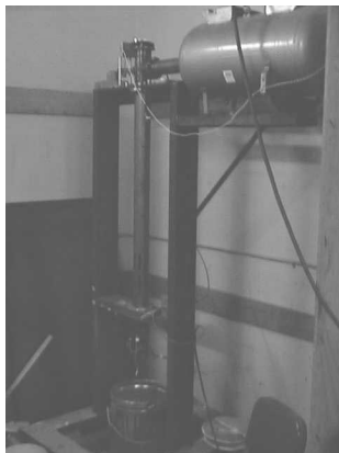
Fig. 8. Airgun at Arizona. The vertical barrel is about 2 m long.
