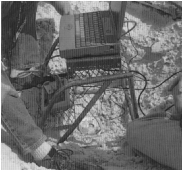
Fig. 14. Downloading the data from the penetrator (disc at lower center). Little or no sand has been removed during the installation of the computer — the impact and/or the airblast excavated the crater seen here (Photo: J. Moersch).
