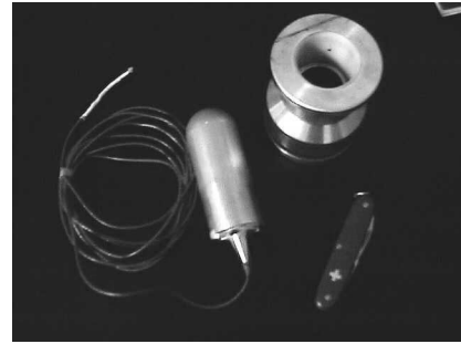
Fig. 9. Projectile components used in test at Arizona. The kevlar-reinforced cable carries the signal from the piezoelectric accelerometer in the back of the cylindrical forebody. The sabot/aftbody is at the upper left; the dark line on the sabot indicates where a pencil lead in the speedometer impacted upon it.
