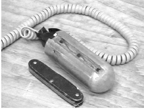
Fig. 11. Photograph of the modified UA penetrator forebody with telephone cord cable and three LM335 sensors.
