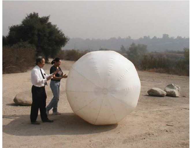
Figure 6. The 6-foot diameter tumbleweed rover used in the magnetometer test at the Arroyo Seco park in Pasadena, California (near the Jet Propulsion Laboratory)
