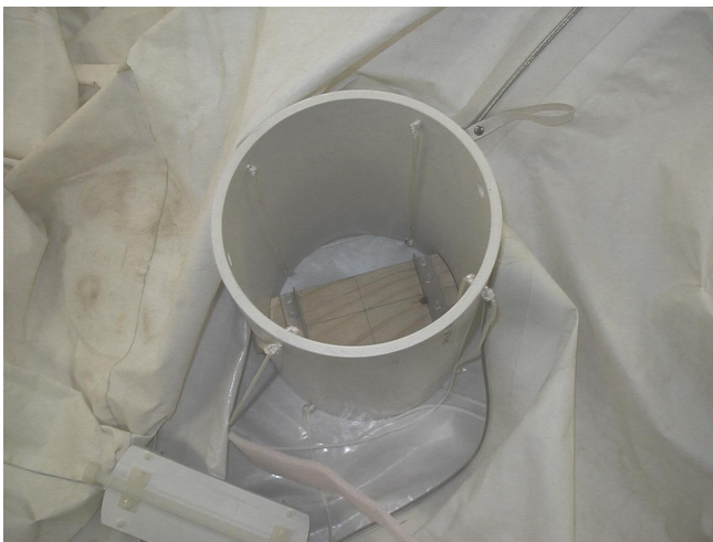
Fig 5. The sensor box was mounted in a central plastic/wood tube (Note the use of nonmagnetic materials!) which was the preferred axis of rotation for the rover. The tube is attached to the fabric of the rover itself via 12 tension cords.
