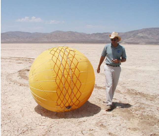
Fig.3 Field test at El Mirage dry lake bed in California of a small-scale tumbleweed rover. Note mesh belt around preferred axis of rotation.
