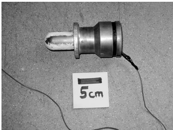
Figure 2. Photograph of the projectile with Kevlar-reinforced coaxial cable. The black band at the rear is a notch for retaining the projectile in the gun barrel with a shear pin. The round-nosed forebody has white paint stripes to record abrasion during penetration.
