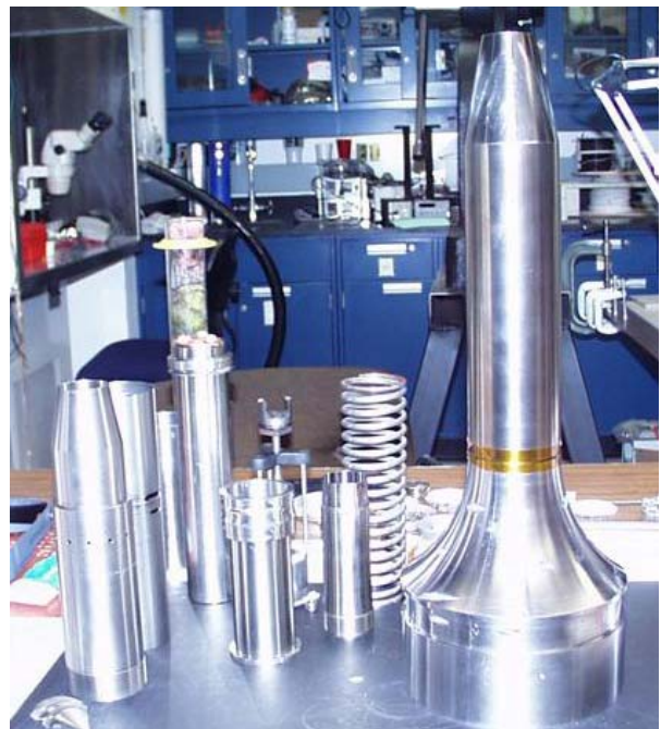
Fig. 4 Some of the internal springs and cylinders making up the sample encapsulation mechanism
