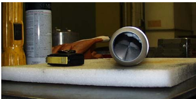
Fig 10. Nose-on view of the sample canister after successful acquisition of an ice target, showing the cruciform arrangement of the four conical nose doors, tightly shut in this instance.
