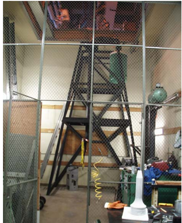
Fig. 6. Airgun facilities at the University of Arizona : behind mesh safety screen is framework supporting main airgun – green airtank at upper right. Ceiling open at top to LPL loading area for insertion of penetrator into breech of gun. On extreme right is small 3-inch gun used in previous experiments. Penetrator is in foreground.
