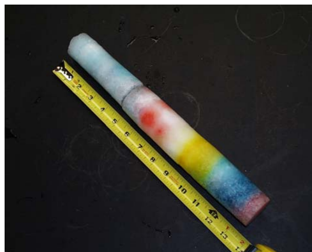
Fig. 12. Ice core recovered from penetrator. Note the narrow section at front, corresponding to the deepest part of the core. Note that the colors of dyed ice layers remain distinct – stratigraphy has been preserved with a vertical resolution comparable with the core diameter.
