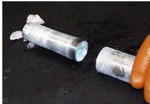
Fig. 11 Opening sample canister – blue-dyed ice inside. Note the thick orange rubber glove and frosting on the canister body – the sample is still at \sim -60^{\circ}\text{C} .
