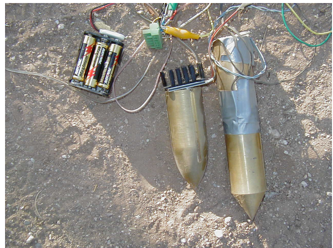
Figure 2. The two test articles prior to emplacement in the ground. A set of AA cells provided excitation for the temperature sensors and the offset voltage required to push the thermoelectric output into the range acquired by the datalogger.
