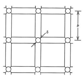
Show that the porosity of such a rock is:  $\phi = \frac{3\pi}{4} \left(\frac{\delta}{b}\right)^2$
