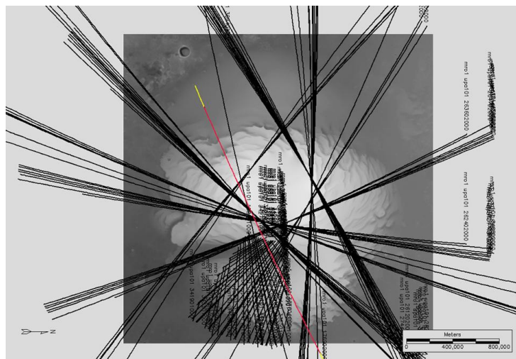
Figure 1: Martian North Polar Region showing array of SHARAD paths. Trace in red is line used in this study. The white region approximates the extent of the icecap – the focus of this research. Reproduced from SHARAD data base map courtesy of Prof J. Holt, University of Texas.
