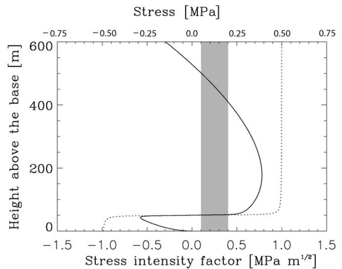
Fig. 5. Extent of penetration of a bottom crevasse above the base of the ice shell as a function of the stress intensity factor (solid line) for a compressive stress at the base and a tensile stress in the middle of the crack (dotted line). The gray area corresponds to fracture toughness for ice that range between  $0.1\text{--}0.4 \text{ MPa m}^{1/2}$ .
