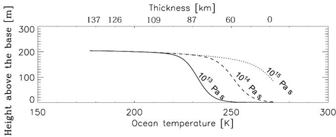
Fig. 4. Height above the base of the ice shell of bottom crevasses as a function of the basal temperature and thickness of the ice shell. The initial ammonia concentration of the ocean is 5%, the ice density is  $917 \text{ kg m}^{-3}$ , and the viscosity of the ice at the melting temperature is  $10^{13} \text{ Pa s}$  (solid line),  $10^{14} \text{ Pa s}$  (dashed line), and  $10^{15} \text{ Pa s}$  (dotted line).
