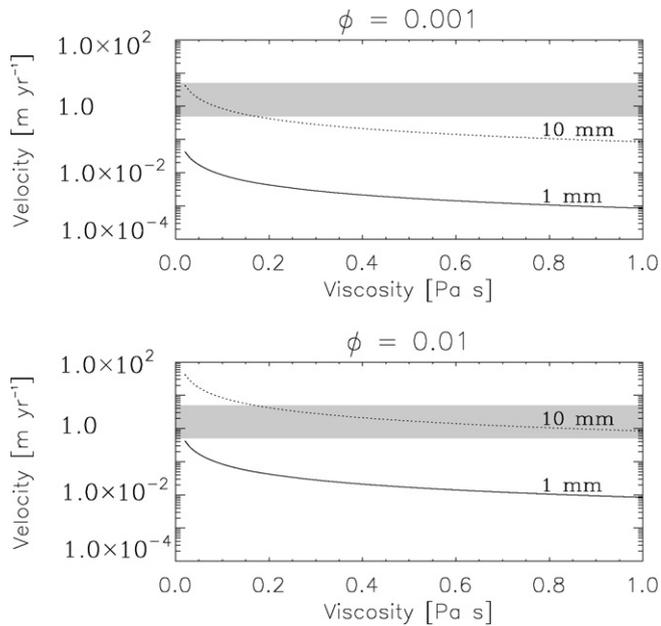
Fig. 7. Percolation velocity through the ice shell of an ammonia water mixture versus the viscosity, and the ice grain size (1 mm in solid lines, 10 mm in dotted lines). The difference in density between the liquid and the ice is  $20 \text{ kg m}^{-3}$ . The plots are for two melt fractions:  $\phi = 0.001$  and  $\phi = 0.01$ . Grey areas show the convective velocity of the ice ( $0.5\text{--}5 \text{ m yr}^{-1}$  range).
