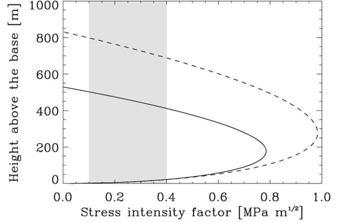
Fig. 3. Stress intensity factor as a function of the height above the ice shell. The tensile stress is  $5 \times 10^4$  Pa and difference in density between the ocean fluid and the ice is  $70 \text{ kg m}^{-3}$ . The solid line shows the crack height in a field of closely spaced crevasses; the dashed line shows the crack height above the base of the ice shell for an isolated crevasse. The gray area corresponds to fracture toughness for ice that range between 0.1 and 0.4  $\text{MPa m}^{1/2}$ .
