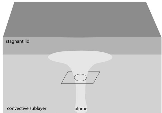
Fig. 1. The model examines a two-dimensional horizontal section of a convective ice shell representing a cross section through a vertically oriented convective plume.
