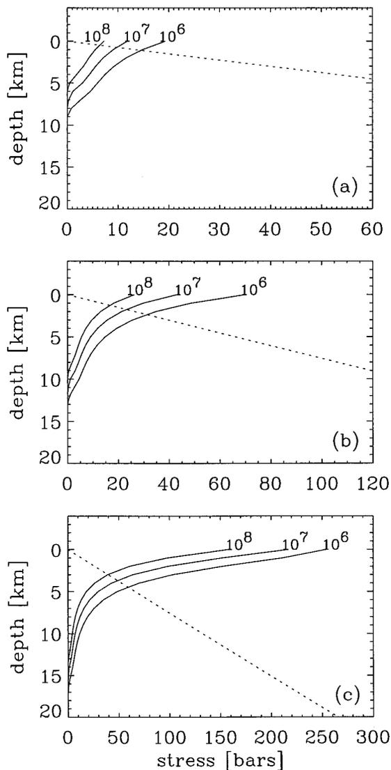
**FIG. 10.** Lithospheric stress versus depth occurring for a volume expansion of 2%, using flow parameters of Durham *et al.* (1992), for the expansion times shown in the plots (years). Assumes  $dT/dz = 5 \text{ K km}^{-1}$ . Dotted line is hydrostatic pressure. (a) Surface  $T = 130 \text{ K}$ , (b) surface  $T = 110 \text{ K}$ , (c) surface  $T = 90 \text{ K}$ . Note the different horizontal scales. The stresses shown imply cracking to several kilometers depth during a large thermal runaway.
