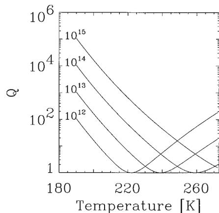
FIG. 3. Ice  $Q(T)$  used in thermal model, as determined by the Maxwell model, Eqs. (2) and (3). We use  $A = 26$ , and show four curves, for  $\eta_0$  from  $10^{12}$  to  $10^{15}$  Pa sec.
