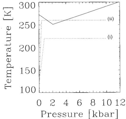
FIG. 2. The water ice melting curve used in the Ganymede thermal model (solid line). Overlain on the melting curve we show two sample model temperature profiles (dotted lines). Each contains a conductive lithosphere and thermal boundary layer, underlain by an isothermal convective region. Case (i) corresponds to a solid Ganymede and case (ii) represents a Ganymede with an internal liquid ocean bounded above and below by ice layers.
