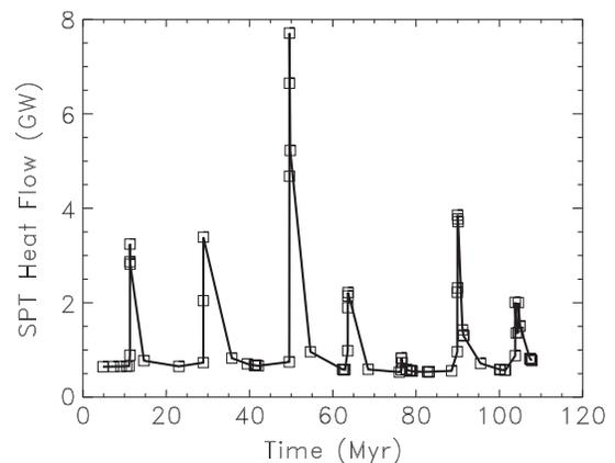
**Figure 4.** SPT heat flow over time in the simulation from Figure 3. Heat flow is integrated over the region south of  $60^\circ\text{S}$  latitude. The episodic nature of the heat flow helps to reconcile the current high heat flow with orbital and evolutionary constraints on Enceladus’ time-integrated power budget.
