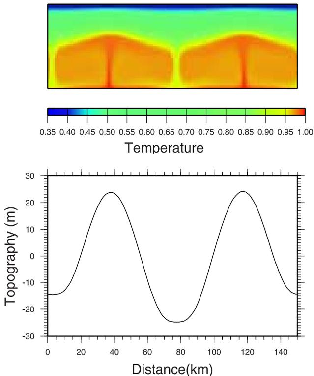
**Figure 5.** (top) Temperature divided by melting temperature for a simulation in a domain 150 km wide and 50 km deep with a melting-temperature viscosity of  $10^{14}$  Pa s. The viscosity contrast is  $10^8$ , tidal flexing amplitude  $\epsilon_0 = 2 \times 10^{-6}$ , basal Rayleigh number is  $4.3 \times 10^7$ , and resolution is  $150 \times 50$ . (bottom) Dynamic topography for the same simulation.
