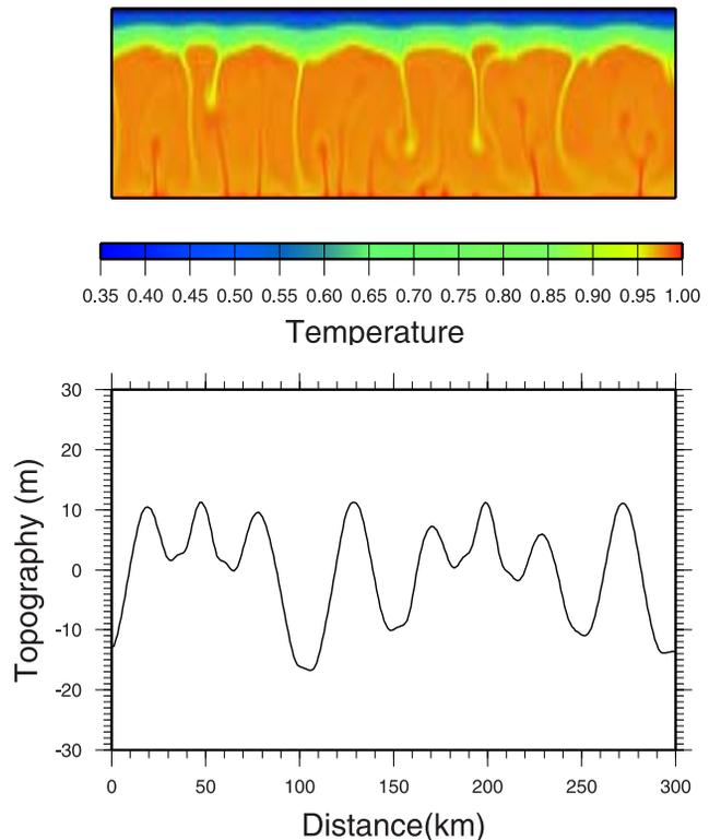
**Figure 2.** (top) Temperature divided by melting temperature for a simulation in a domain 300 km wide and 50 km deep. The viscosity contrast is  $10^9$ , melting-temperature viscosity is  $10^{13}$  Pa s, constant tidal heating is  $q = 1 \times 10^{-7} \text{ W m}^{-3}$ , basal Rayleigh number is  $4.3 \times 10^8$ , and resolution is  $300 \times 50$  in the horizontal and vertical directions. (bottom) Dynamic topography for the same simulation.
