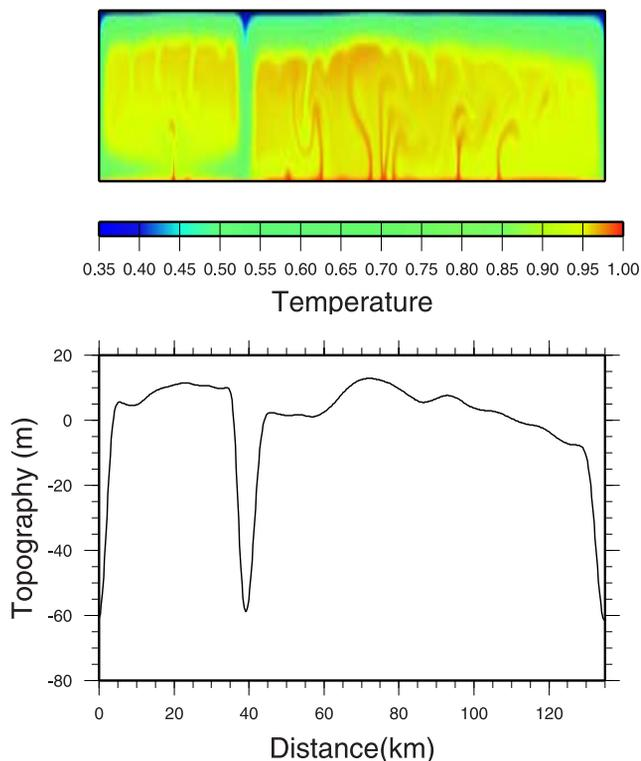
**Figure 6.** (top) Temperature divided by melting temperature for a simulation in a domain 135 km wide and 15 km deep with a melting-point viscosity of  $10^{12}$  Pa s. The viscosity contrast is  $10^4$ , constant tidal heating is  $q = 1 \times 10^{-6} \text{ W m}^{-3}$ , basal Rayleigh number is  $1.2 \times 10^8$ , and resolution is  $450 \times 50$  in the horizontal and vertical directions. (bottom) Dynamic topography for the same simulation.
