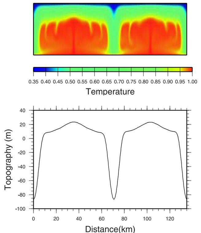
**Figure 4.** (top) Temperature divided by melting temperature for a simulation in a domain 135 km wide and 15 km deep. The melting-point viscosity  $\eta_0$  is  $10^{13}$  Pa s, viscosity contrast is  $10^4$ , basal Rayleigh number is  $1.2 \times 10^7$ , and resolution is  $450 \times 50$  in the horizontal and vertical directions. Tidal heating is temperature-dependent with tidal-flexing strain amplitude  $\epsilon_0 = 2 \times 10^{-5}$ . (bottom) Dynamic topography for the same simulation.
