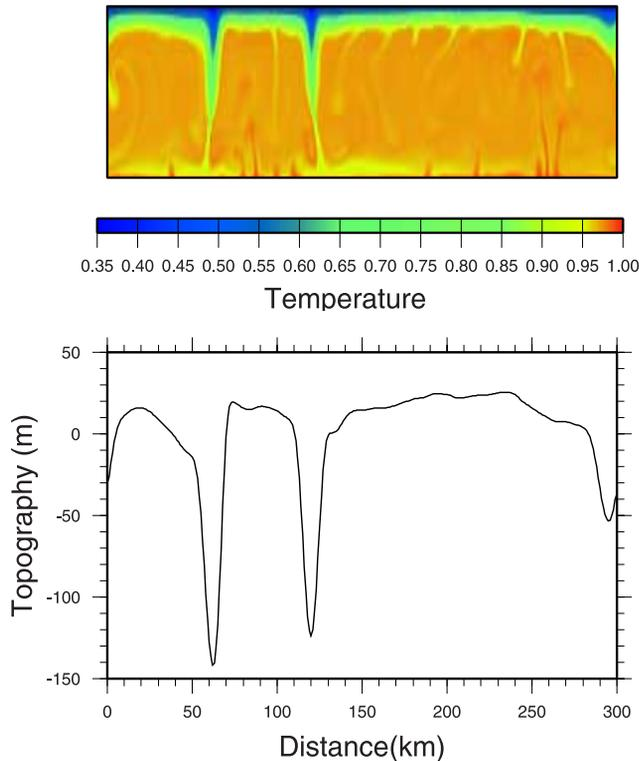
**Figure 3.** (top) Temperature divided by melting temperature for a simulation in a domain 300 km wide and 50 km deep. The melting-point viscosity  $\eta_0$  is  $10^{13}$  Pa s, viscosity contrast is  $10^4$ , constant tidal heating rate is  $3 \times 10^{-7}$  W m $^{-3}$ , basal Rayleigh number is  $4.3 \times 10^8$ , and resolution is  $300 \times 50$  in the horizontal and vertical directions. (bottom) Dynamic topography for the same simulation.
