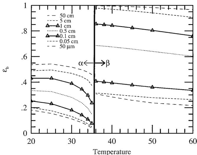
**FIG. 2.** The Planck-mean bolometric emissivity of  $N_2$  ice as a function of temperature and particle size. The double vertical line marks the  $\alpha$ - $\beta$  phase transition temperature at 35.6 K. The dotted lines show the emissivity for nominal grain sizes deduced from visible and near-IR spectroscopy of Pluto and Triton. Reproduced from Fig. 3 of Stansberry *et al.* (1996a) with permission from Elsevier Science.
