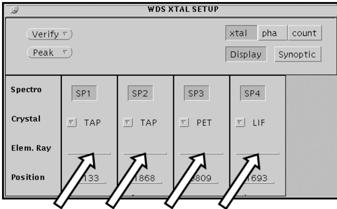
**R-Click for each spectrometer and select the correct reference X-ray line from the periodic table.**
