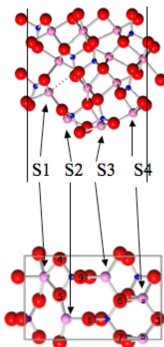
Figure 3 Illustrations of the {100} surface, where red, pink and blue represent oxygen, magnesium and silicon atoms respectively; the top illustration is a schematic representation of a part of the olivine slab viewed perpendicular to the surface (bottom side of the slab) and the bottom illustration represents view parallel to the surface unit cell. “Sn” identifies the possible adsorption sites, where “n” denotes the nth adsorption site.
