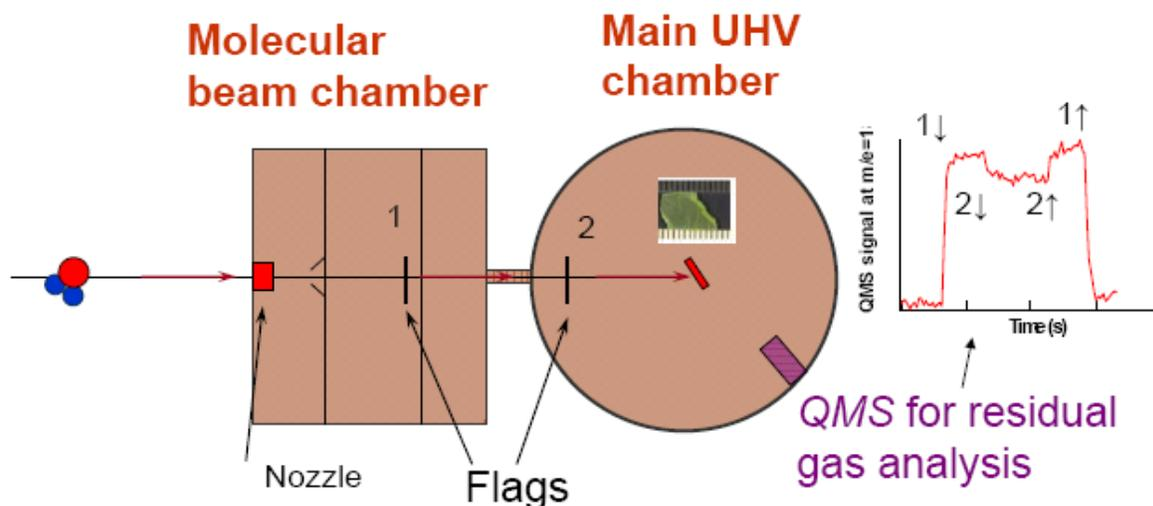
**Figure S1: Schematic drawing of the Supersonic Molecular beam chamber coupled to the ultra high vacuum chamber (Main UHV chamber).** The UHV chamber contains an olivine sample (see photo in the inset) and equipped with a quadrupole mass spectrometer (QMS) for residual gas analysis. The latter is used for King and Well's measurements of the sticking probability (see text).
