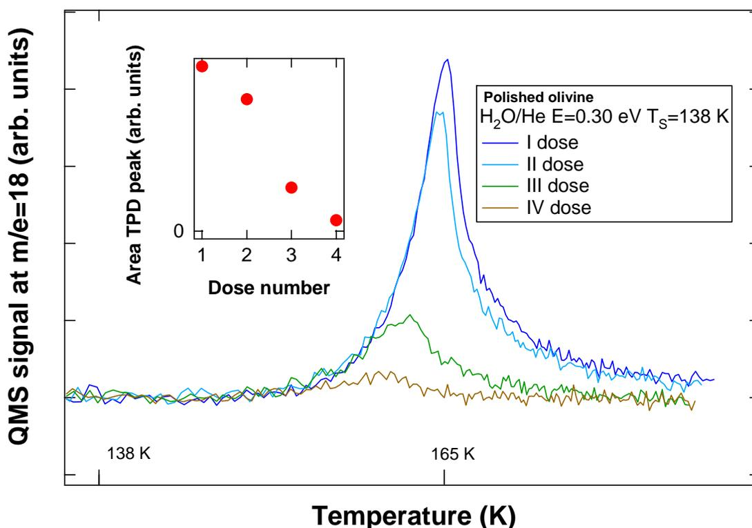
Figure 1 **Temperature Programmed Desorption (TPD) spectra from the {100} olivine surface for repeated identical doses (600 s) of water at 138 K.** The highest intensity peak corresponds to desorption of molecularly adsorbed water in multilayers. Prior to performing a new dose, the sample was prepared by heating the crystal well above the desorption temperature of molecularly adsorbed water (165 K). The lower signal observed for the subsequent doses
