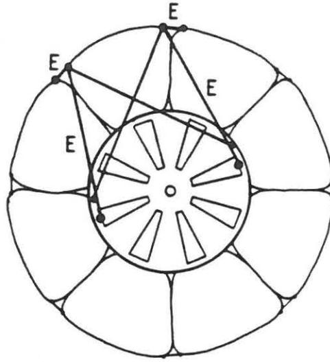
**Figure 5.4.** Several of the configurations of elastic cords, **E**, used to align sectors.
