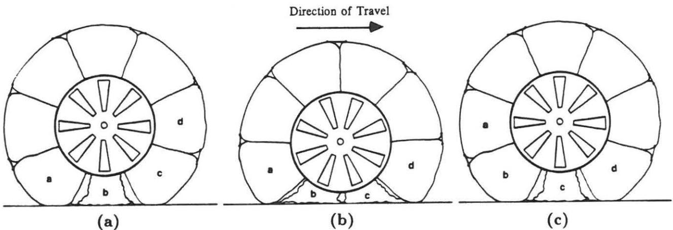
**Figure 2.2.** Mars Ball rolling sequence. (a) Position of sectors at the start of a forward motion sequence. (b) Position of sectors after deflation of forward sector 'c'. (c) Position of sectors after inflation of sector 'b'. The wheel has now completed one-eighth of a revolution and has returned to its original configuration.
