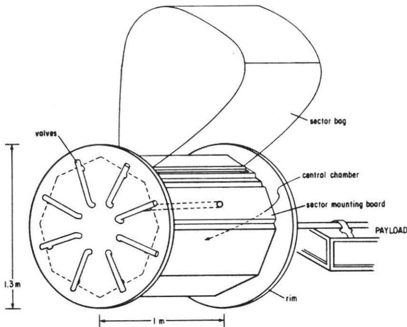
**Figure 4.1a.** Schematic of Phase II hub construction.
