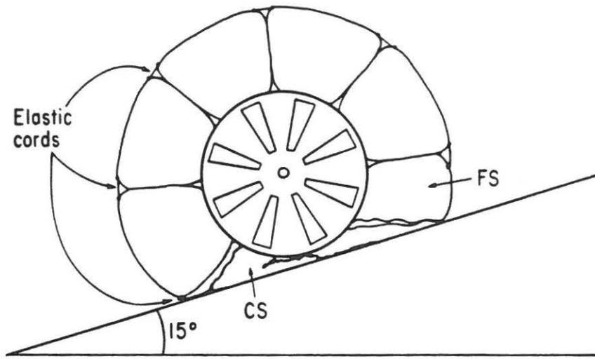
**Figure 5.3.** Limitation to slope-climbing by the Phase II Mars Ball. When negotiating slopes the critical sector, **CS**, could become pinched beneath the hub, preventing further progress. **FS** refers to the front sector.
