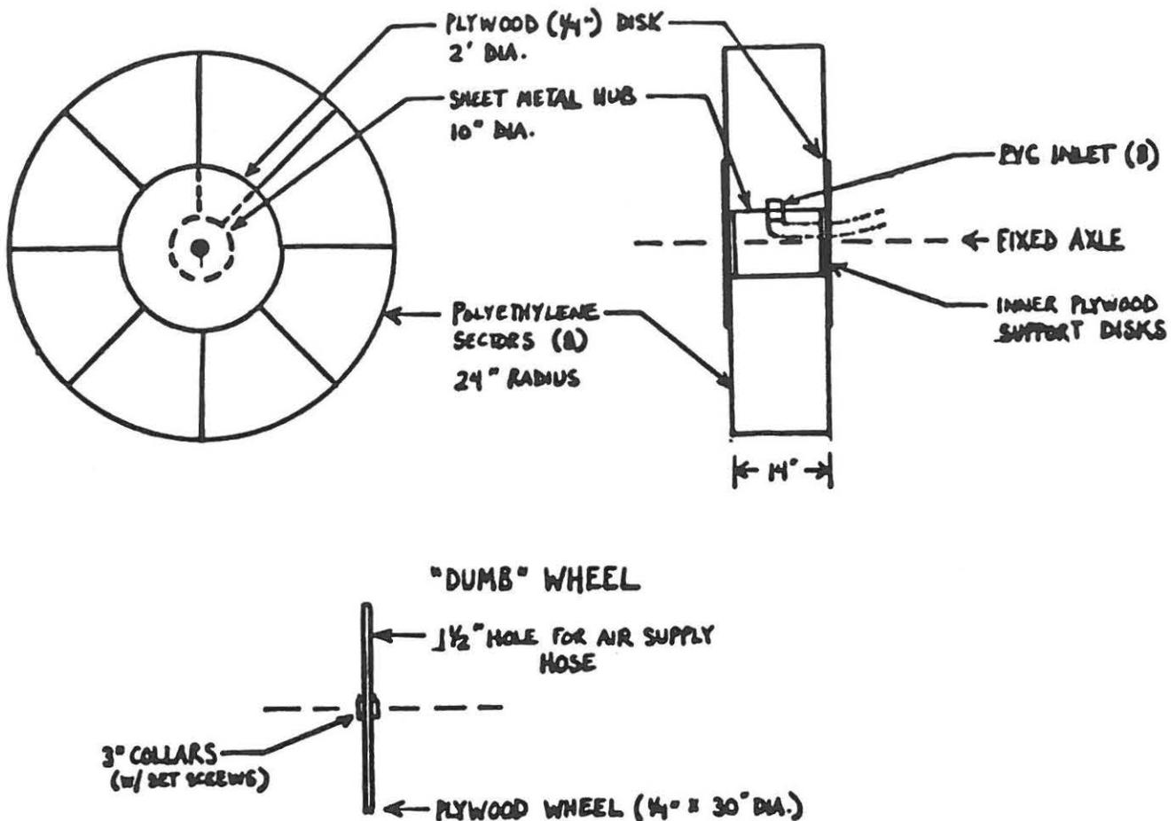
Figure 3.1a. Schematic of Phase I wheel construction. "Dumb" wheel occupies one end of a central axle and supplies support only.
