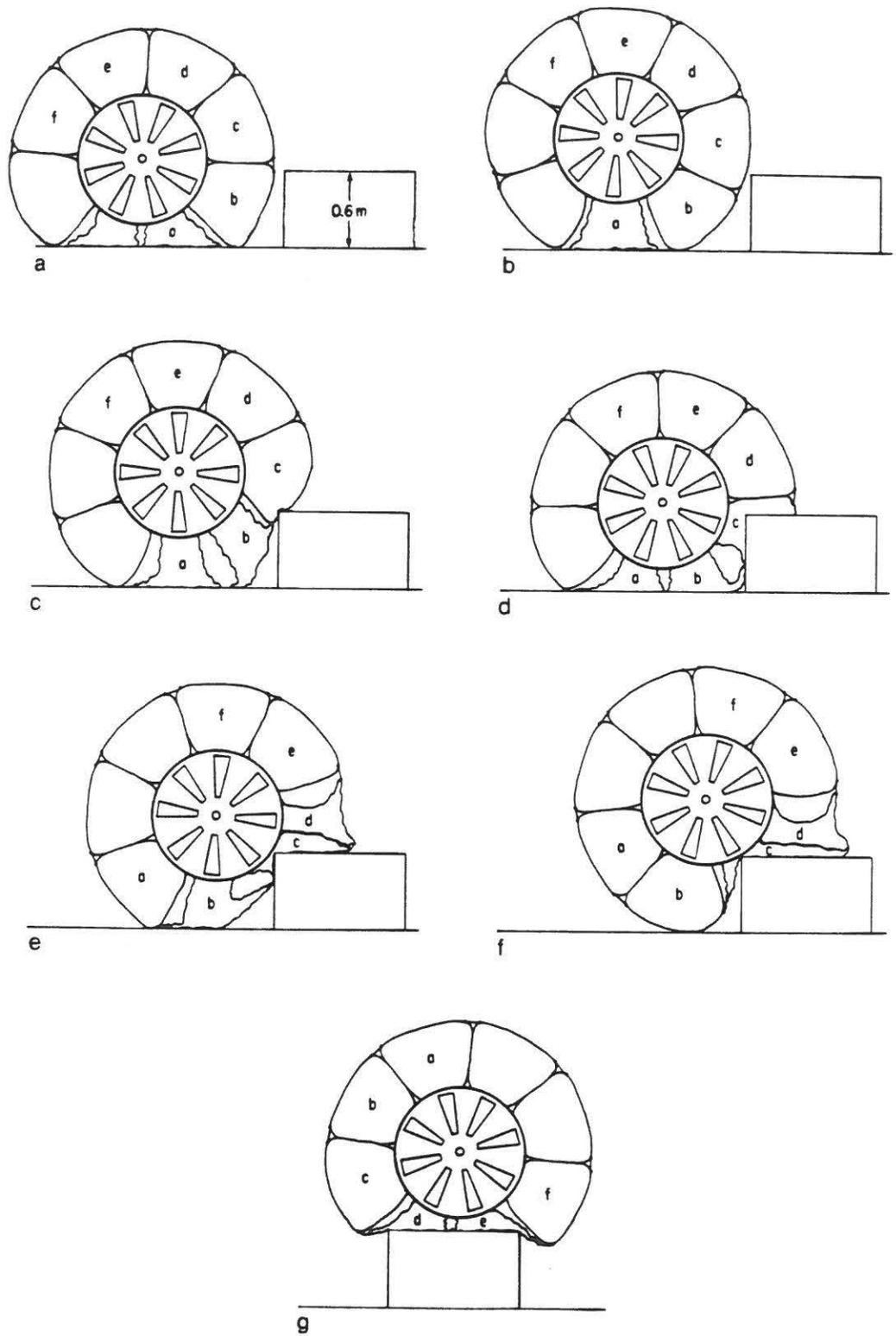
Figure 5.7. Mars Ball obstacle-climbing sequence.
