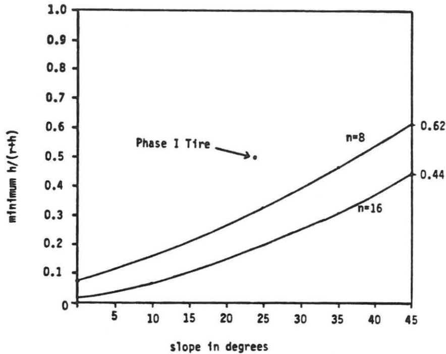
**Figure 2.4.** Inflatable fraction of the wheel necessary to climb a given slope. Curves are for ideal wheels with 8 and 16 sectors. Actual performance of the Phase I wheel is plotted.
