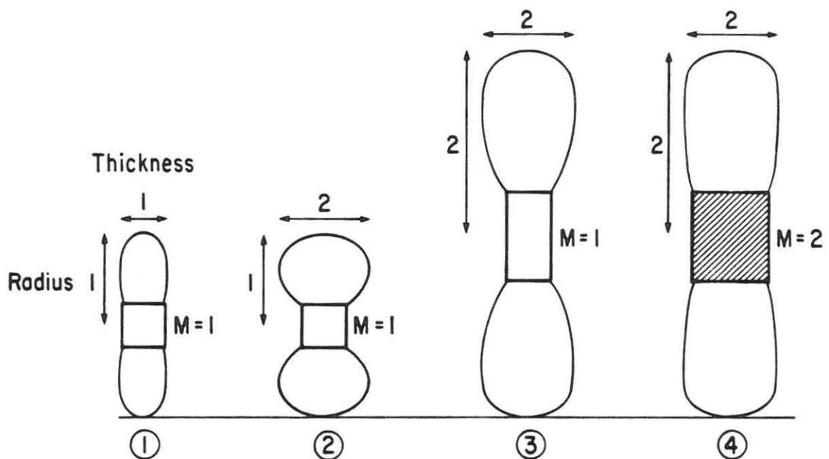
**Figure A3.** Cross sections of possible alternative wheel designs. Case 1 is the current wheel whose dimensions are taken as unity in the discussion.
