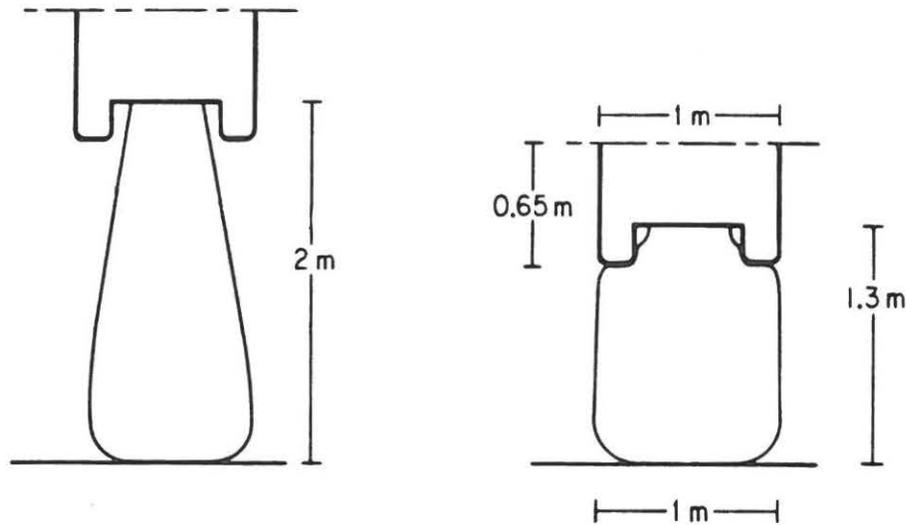
Figure 5.2. Comparison of size and shape of long 2 m and short 1.3 m bags.
