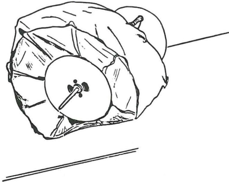
**Figure 3.3.** Slope-climbing by Phase I Mars Ball.
