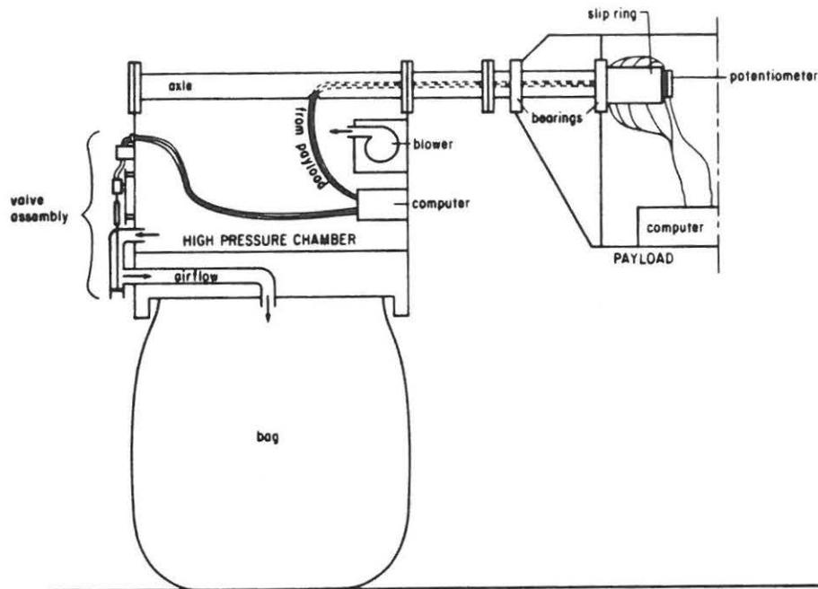
Figure 4.1b. Profile through Phase II hub and axle.
