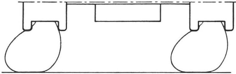
**Figure 5.1a.** Lateral instability experienced with the Phase II vehicle.
