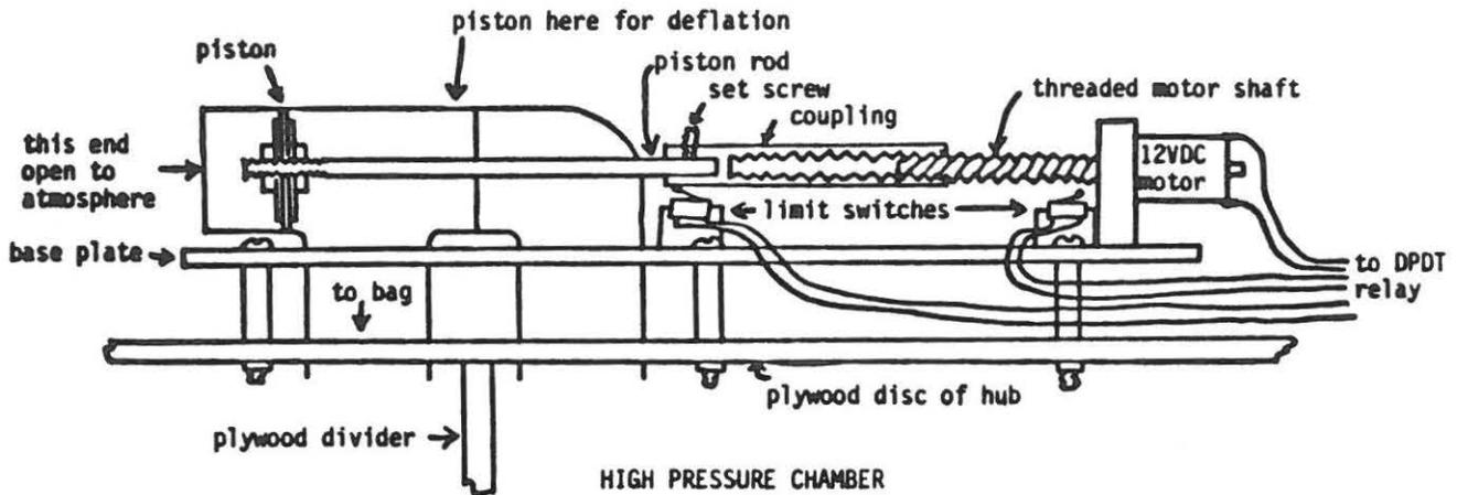
Figure 4.2. Valve assembly for Phase II Mars Ball.
