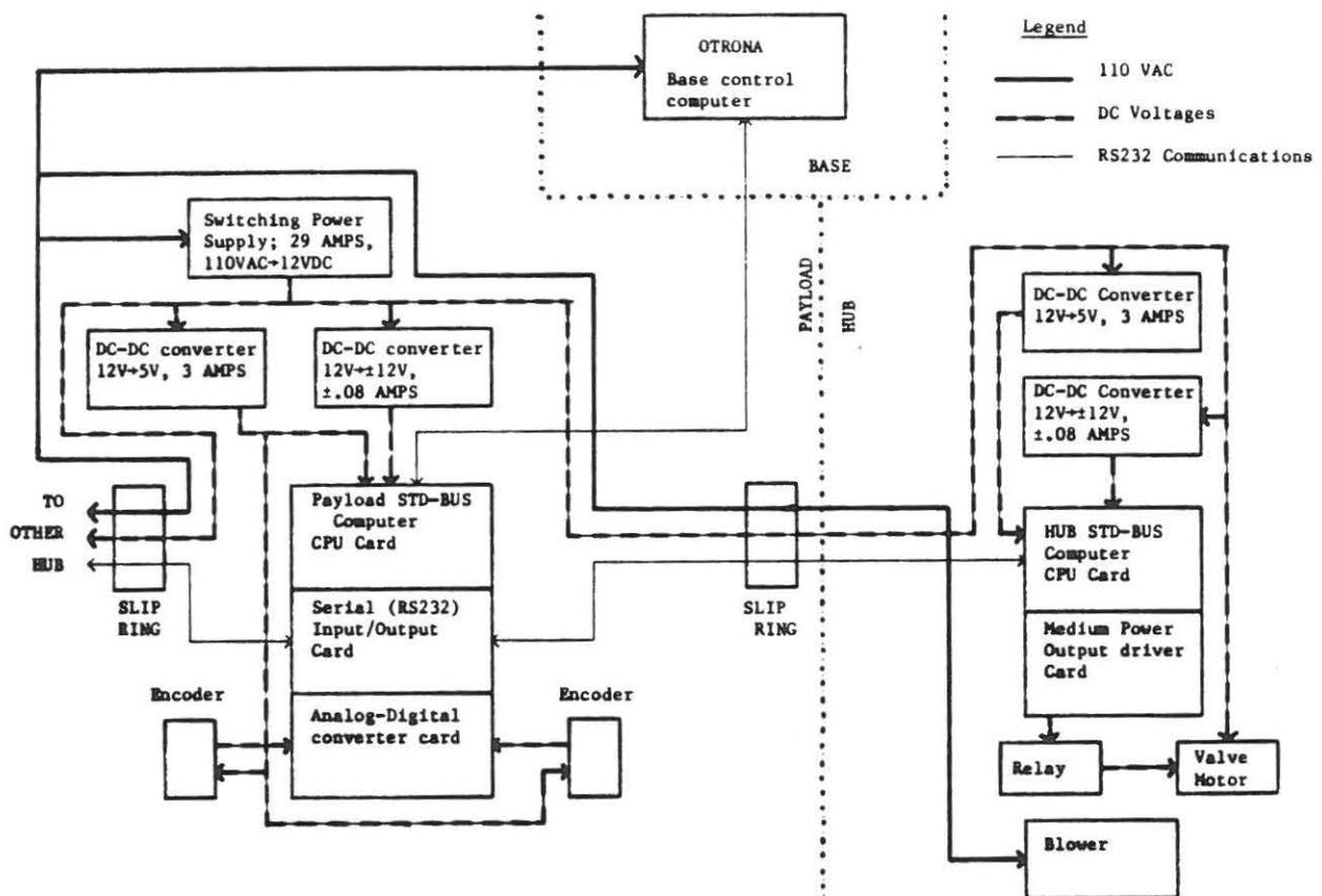
Figure 4.6. Power and communications distribution circuitry.
