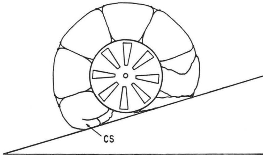
**Figure 5.5.** A second limitation to slope-climbing by the Phase II vehicle. The distorted critical sector, **CS**, did not push the hub uphill.
