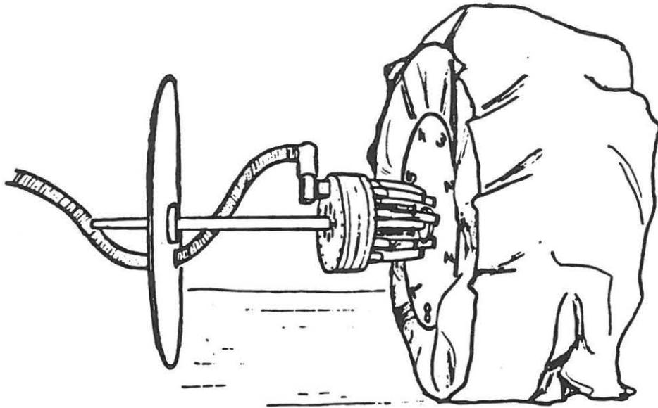
**Figure 3.2.** Completed Phase I Mars Ball. Pressurized air is supplied by an off-board compressor through the tube running off to the left.
