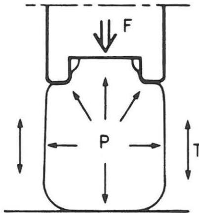
**Figure 5.1b.** Important forces affecting stability. The weight of the vehicle provides a downward force,  $F$ , opposed by the bag pressure,  $P$ . Bag tension,  $T$ , helps maintain bag shape.
