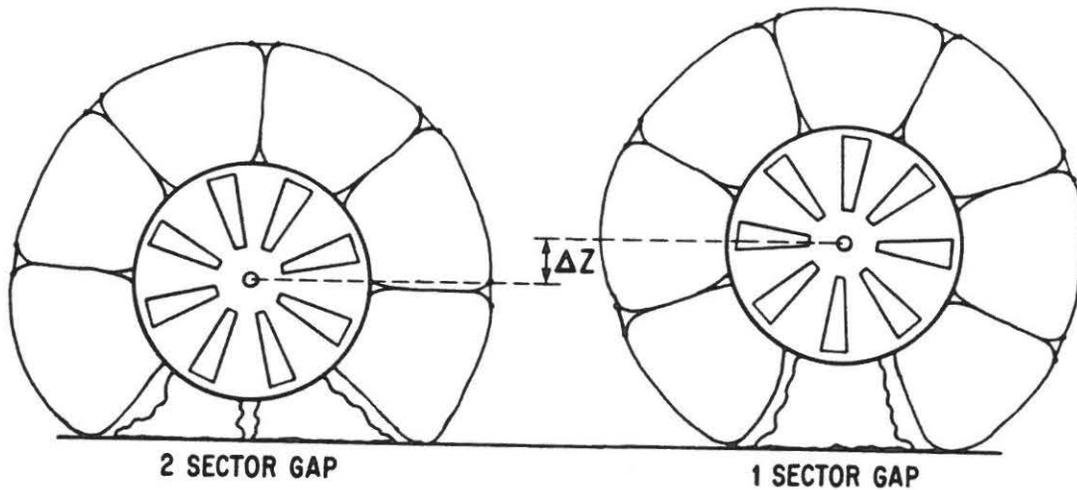
Figure A1. Work done against gravity in vertical motion of the Mars Ball.
