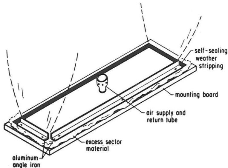
Figure 4.3. System for mounting inflatable sectors to the hubs.
