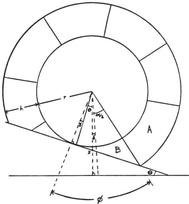
**Figure 2.3.** Idealized climbing geometry of a Mars Ball wheel. Refer to text for labels and discussion.
