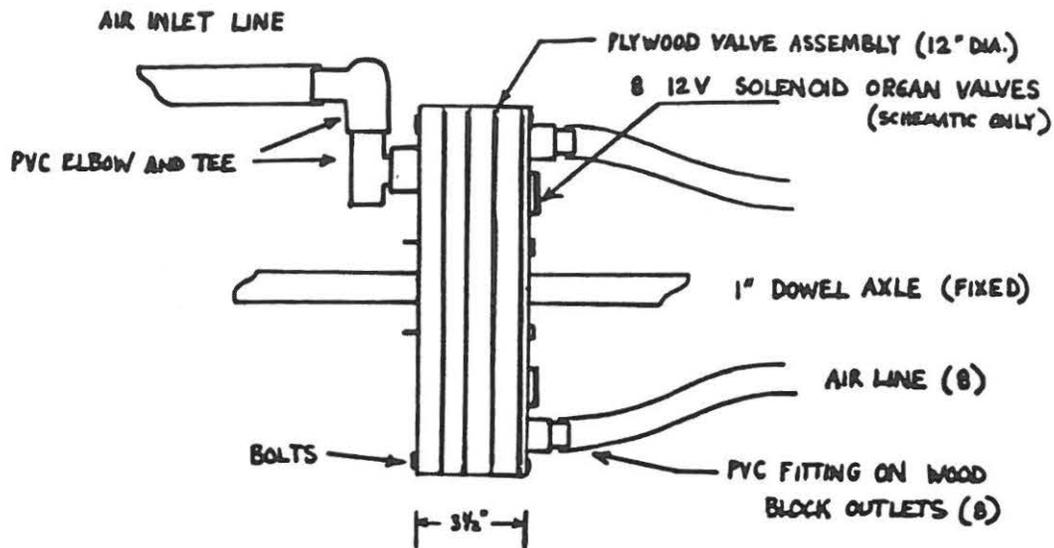
Figure 3.1b. Details of Phase I hub, valves and air supply.
