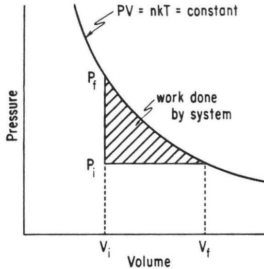
Figure A2. PdV work done during inflation of sectors.
