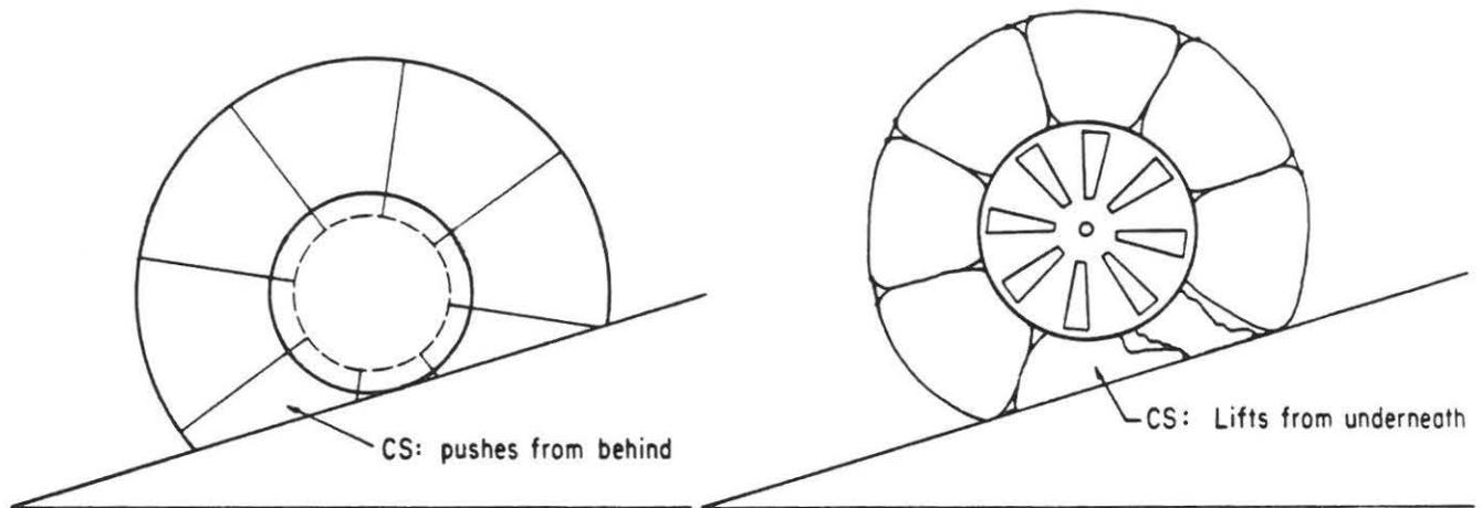
**Figure 5.6.** Comparison of manners of slope-climbing by the Phase I (left) and Phase II (right) vehicles. The critical sector, CS, in the Phase II prototype was frequently trapped beneath the hub, and inflation tended to lift the vehicle until it fell forward. The Phase I critical sector was better positioned to roll the wheel uphill by pushing from behind.
