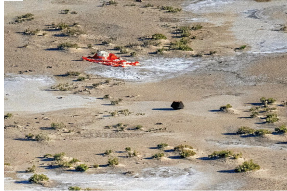
The sample-return capsule from University of Arizona-led OSIRIS-REx mission rests in the Utah desert near its main parachute, shortly after touching down on Sept. 24. A new NASA report details a problem with the capsule's smaller drogue chute during the landing. KEEGAN BARBER, NASA
