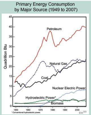
U.S. energy supply is dominated by fossil fuels. Petroleum, the top source of energy shown above, is primarily used for transportation (70 percent of oil use). Natural gas is used in roughly equal parts to generate electricity, power industrial processes, and heat water and buildings. Coal is primarily used to generate electricity (91 percent of coal use). Nuclear power is used entirely for electricity generation.
