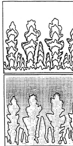
Figure 10a. Plan view of a simulated valley network that formed in an experimental sapping chamber with a flow of discharge of 10 cm 3 s -1 . The scale shows the positions of the river at the outlet at intervals of 25 mm. (b) View from above showing the flow field at the outlet of the chamber after 100 min. Arrows are assumed to be at zero length within the valleys.
