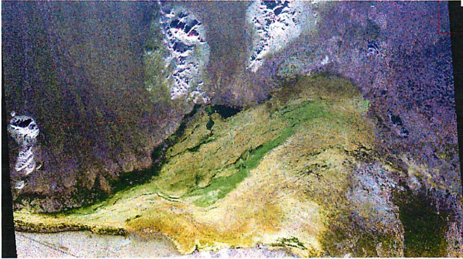
Figure 4: The left figure shows P (80 cm) band HH in the red channel, P band VV in the green channel, P band HV in the blue channel. The center figure shows L (25 cm) band HH in the red channel, L band VV in the green channel, L band HV in the blue channel. The right figure shows C (5 cm) band HH in the red channel, C band VV in the green channel, C band HV in the blue channel. In the L and C bands all the scattering from the plays is surface scattering. In the P band you have some volume scattering (blue).
