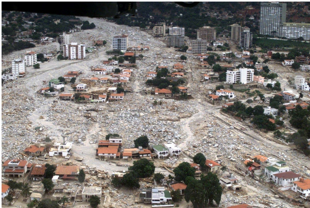
Above: The extent of mudflows in a small part of Vargas, Venezuela. Large boulders carried by the flows helped to cause major damage.
