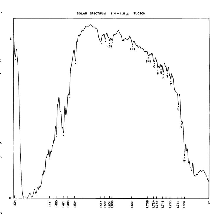
Fig. 8. Photographic reproduction of solar spectrum serving as comparison spectrum for  $\alpha$  Orionis, shown in Figure 7. Nearly all features shown are due to  $H_2O$ ; four dips near G are due to atmospheric  $CO_2$ .
