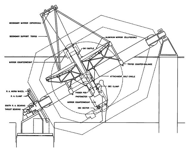
Fig. 2a. Preliminary design for a 10 ft. IR telescope, used at Cassegrain focus. Dotted line shows fork in 6-hour East position.
