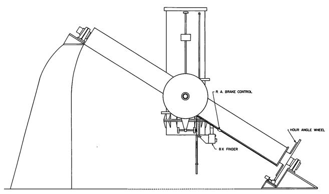
Fig. 3a. Design drawing of 21-inch telescope by W. L. Richards Co. of Austin, Texas, manufacturers of this instrument.
