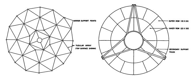
Fig. 2b. Left: Plan view of mirror support truss; each intersection provides collimation for one or more mirrors. Right: Plan view of mosaic mirror and secondary support system.
