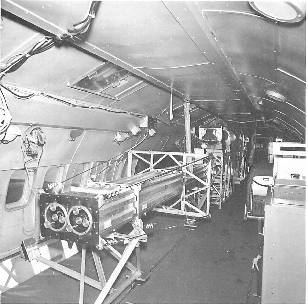
Fig. 1a 4.2-meter solar spectrometer in NASA CV-990 Jet, with 12-inch feeder telescope beyond. Note shock-mount attachments to seat rail; central extended frame with 8 cables for keeping heavy end-plates of spectrometer parallel. Vertical tube supplying dry outside air to spectrometer seen beyond central frame. Adjustment screws at left, control focus and orientation of collimator and camera mirrors. (NASA Photograph)
