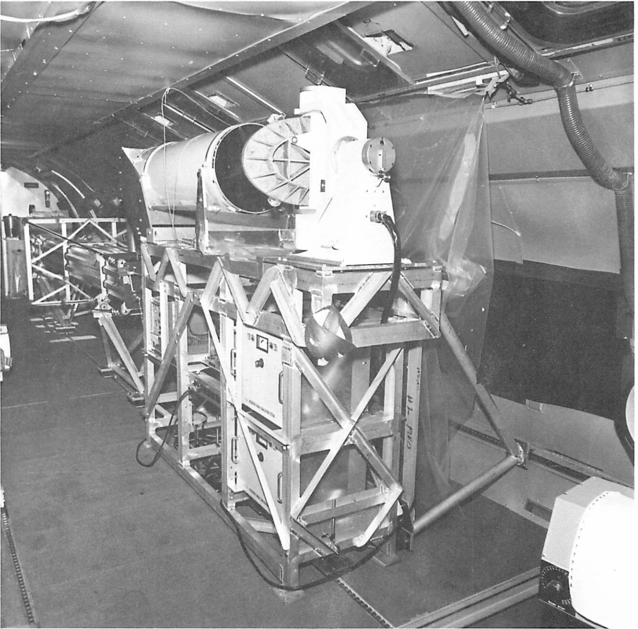
Fig. 1b 12-inch horizontal Cassegrain telescope, fed with heliostat (elliptical mirror in white frame). Control of heliostat gyroscopic, with electronics in rack below. Optical window, with safety covers front and back, above heliostat mount. 4-meter spectrometer beyond, at left. During operations entire unit enveloped in plastic sheet, ventilated with dry outside air. (NASA Photograph)
