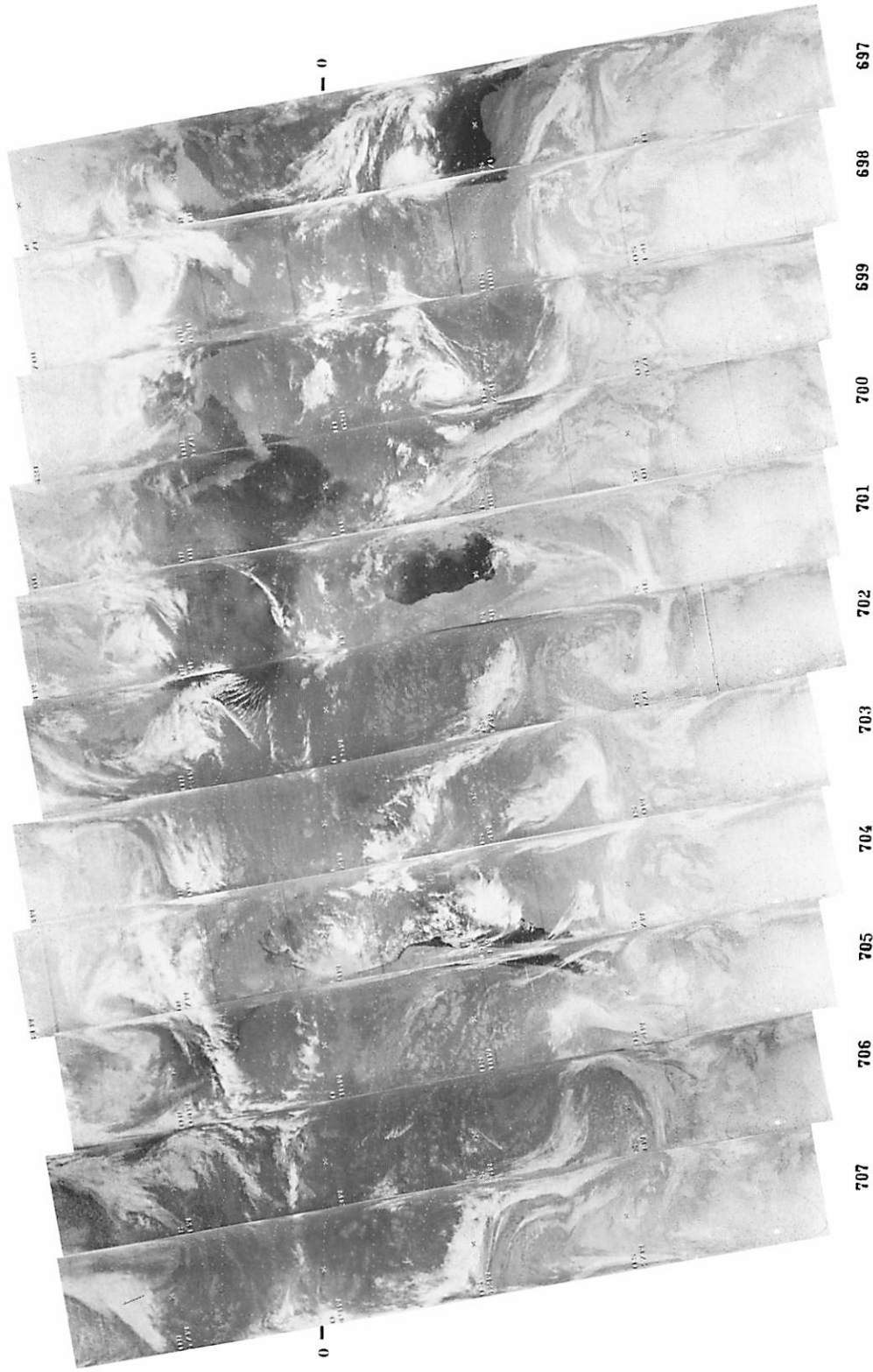
Fig. 6c Montage of 11 consecutive orbital strips taken in window 10-12.5 \mu on Nimbus V, taken simultaneously with Fig. 6a. South America, Africa, Arabia, India, and Australia well shown, with Pacific coastal outline of North America. (Courtesy Dr. W. Nordberg, NASA)
