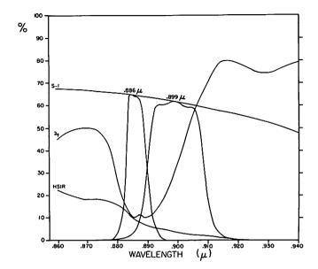
Fig. 3 Relative response of S-1 photo-emissive surface (RCA 6914), with 100% assumed at 0.370µ; Sun/Jupiter intensity ratio for EZ, from Carl Pilcher (1971); relative sensitivity of Kodak HSIR film, with 100% assumed at 0.400µ; and transmission of 0.899µ and 0.886µ filters
