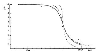
Fig. 7 Estimated light curve of ingress of SAO 159683 and Beta Scorpii with theoretical curves for atmosphere with scale heights of 12 km(short dashes) and 32 km (long dashes)
