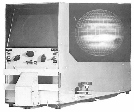
Fig. 7 The projection comparator controls and viewing screen, with the image of Jupiter and grid as seen on the viewing screen
