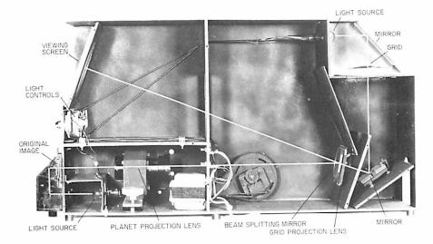
Fig. 8 The interior configuration of the projection comparator
