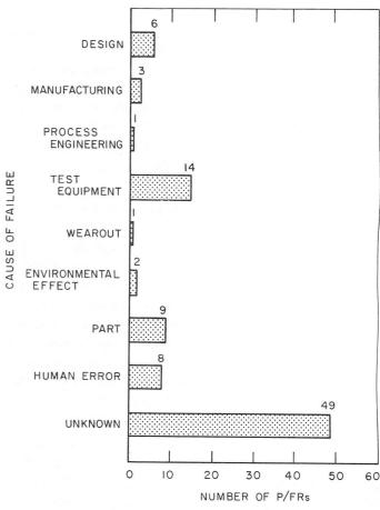
Fig. XII-16. Surveyor alpha scattering instrument problem/failure reports by failure cause
