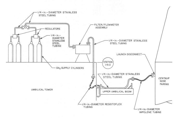
Fig. VIII-19. Alpha scattering instrument gaseous nitrogen purging system
