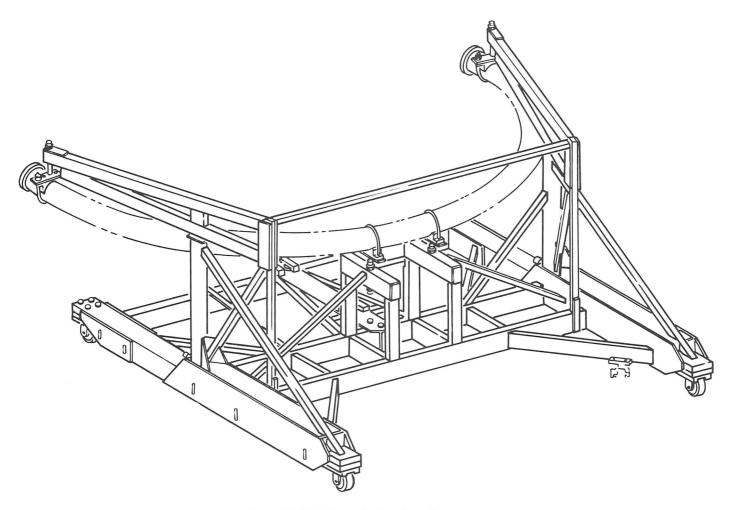
Fig. VIII-28. Nose fairing handling cart
