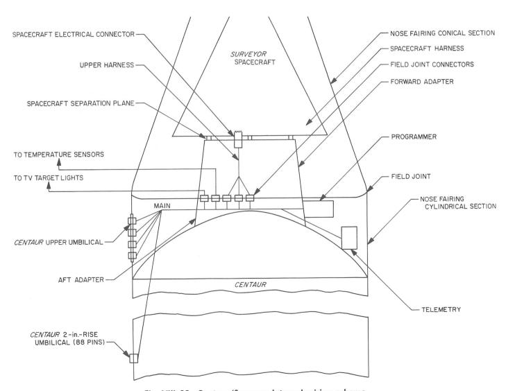
Fig. VIII-23. Centaur/Surveyor internal wiring scheme
