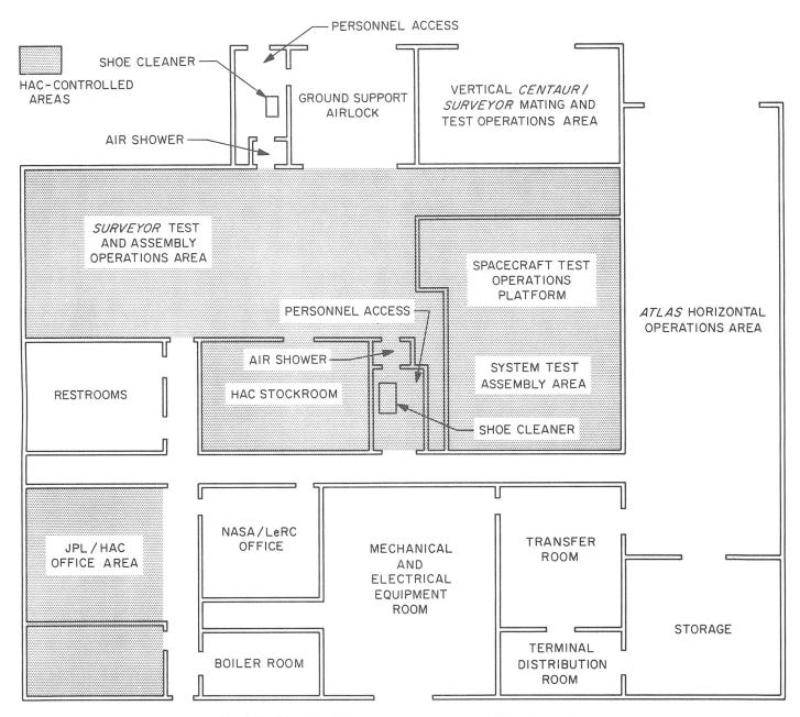
Fig. VIII-21. Combined systems test stand first floor plan
