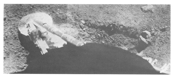
Fig. II-2. Wide-angle mosaic of footpad 2 and the trench formed during Surveyor V landing. The depression formed during the first impact of footpad 2 can be seen at the right-hand end of the trench (September 14, 1967, between 04:00 and 06:00 GMT; Catalog 5-MP-19)
