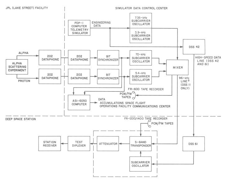
Fig. VII-15. Alpha scattering experiment simulation configuration
