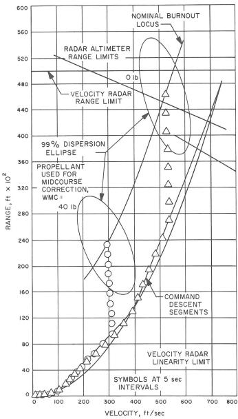
Fig. VI-23. Vernier descent phase (unbraked impact angle: 24 deg)
