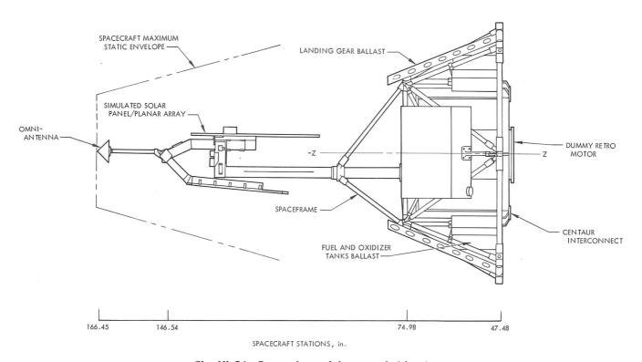
Fig. XI-26. Dynamic model top and side view
