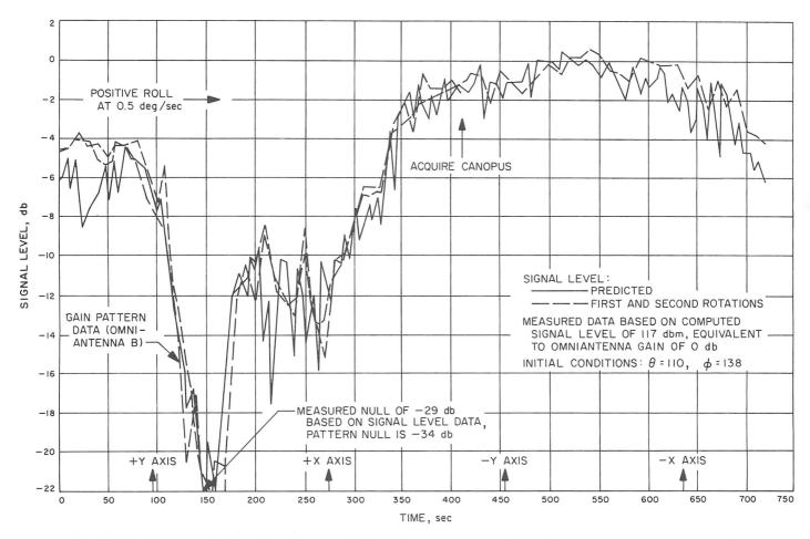
Fig. VI-43. Surveyor III signal level vs predictions during star acquisition for omniantenna B downlink
