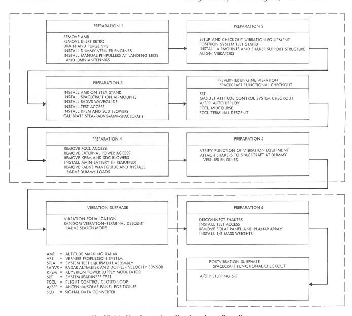
Fig. XI-16. Vernier engine vibration phase flow diagram
