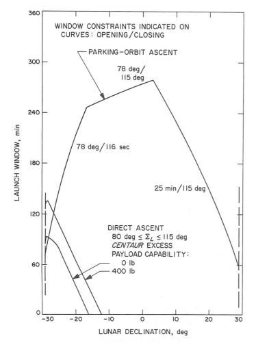
Fig. VI-11. Launch window vs lunar declination
