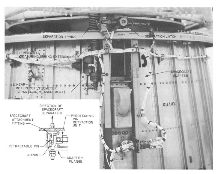
Fig. VIII-12. Payload separation mechanism and instrumentation
