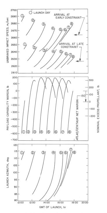
Fig. VI-14. Design chart for typical direct-ascent launch period
