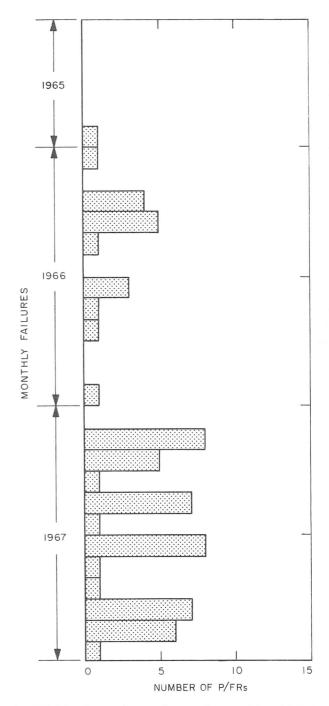
Fig. XII-23. Surveyor vernier engine problem/failure reports by month
