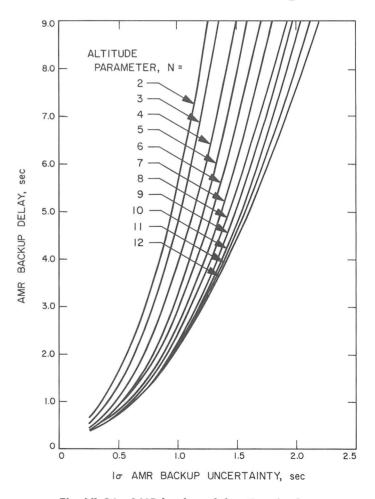
Fig. VI-26. AMR backup delay time (radar reliability: 0.999)
