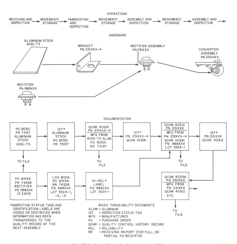
Fig. XII-4. Typical flow—hardware vs traceability
