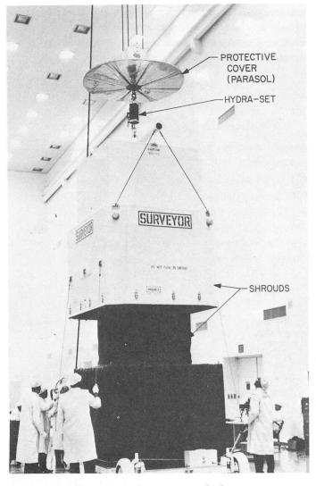
Fig. IX-2. Ground transport vehicle GTV-1
