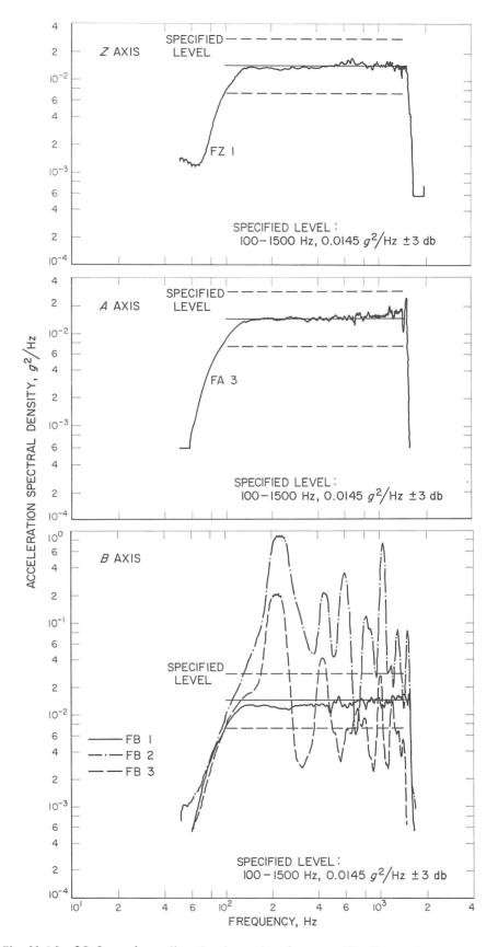
Fig. X-12. SC-3 random vibration input level vs specification values
