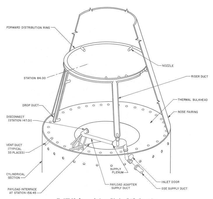
Fig. VIII-10. Spacecraft air-conditioning distribution system
