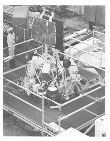
Fig. XI-14. Vibration test setup
