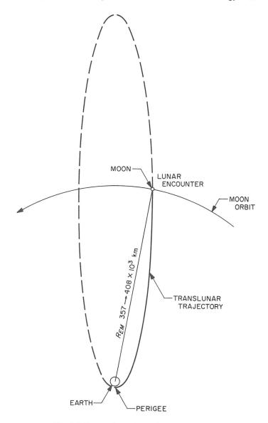
Fig. VI-2. In-plane translunar geometry (approximately to scale)
