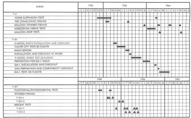
RADVS = RADAR ALTIMETER AND DOPPLER VELOCITY SENSOR
