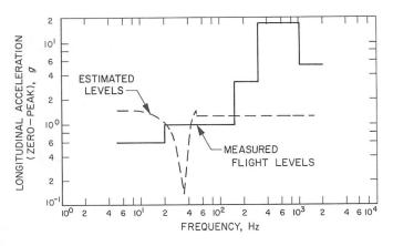
Fig. X-14. Comparison of the 95% flight equivalent sinusoidal vibration environment and the estimated sinusoidal vibration environment for the longitudinal axis
