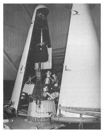
Fig. VIII-16. Spacecraft encapsulation
