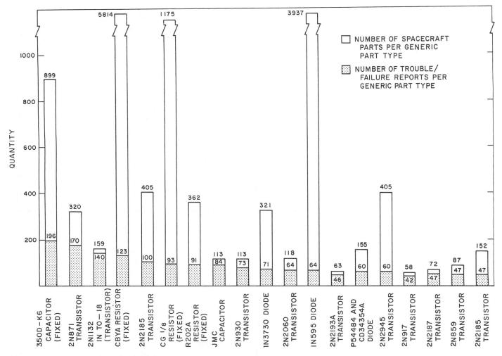
Fig. XII-11. Electronic parts (generic-type) trouble/failure reports
