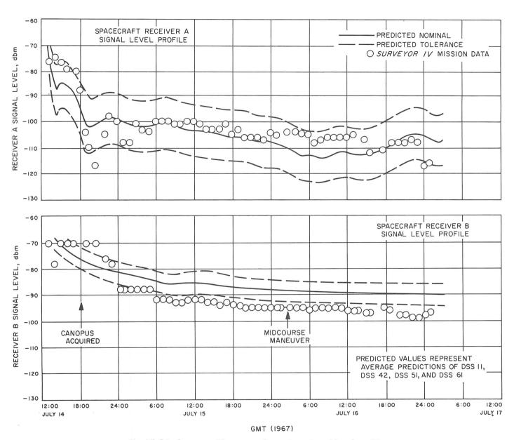
Fig. VI-36. Surveyor IV spacecraft receiver signal level profile
