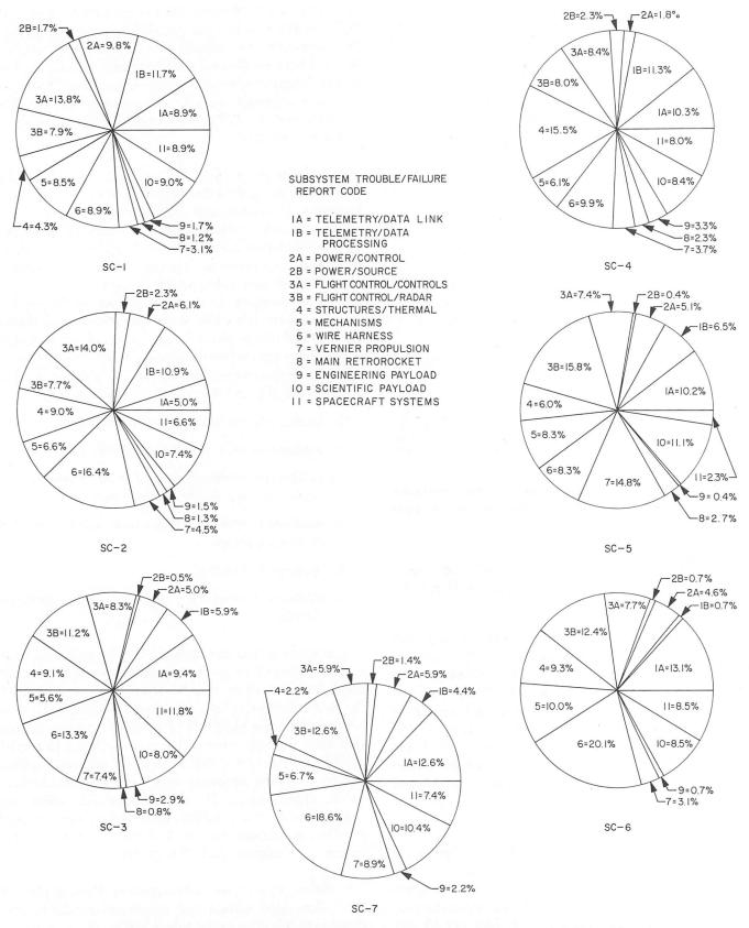
Fig. XII-9. Spacecraft trouble/failure reports by major subsystems (1965 and later)
