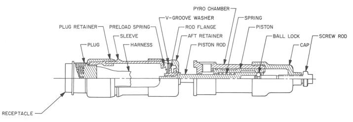
Fig. VIII-13. Electrical connector separation mechanism
