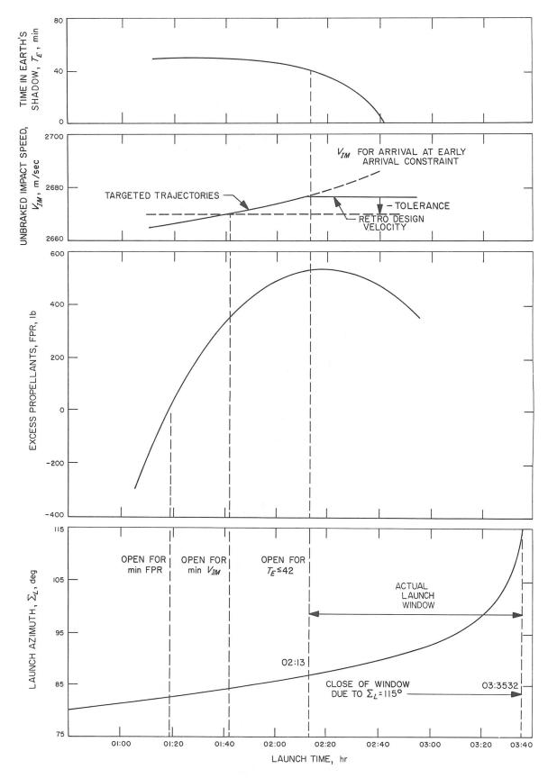
Fig. VI-35. Sample launch window refinement
