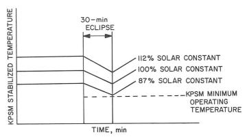
Fig. X-2. Determination of the 87% solar constant test level
