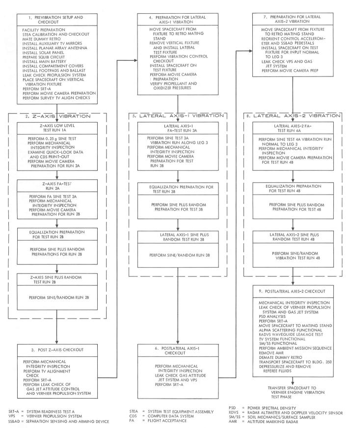
Fig. XI-13. Vibration test phase flow diagram
