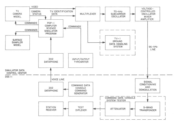
Fig. VII-14. Television/surface sampler simulation system configuration
