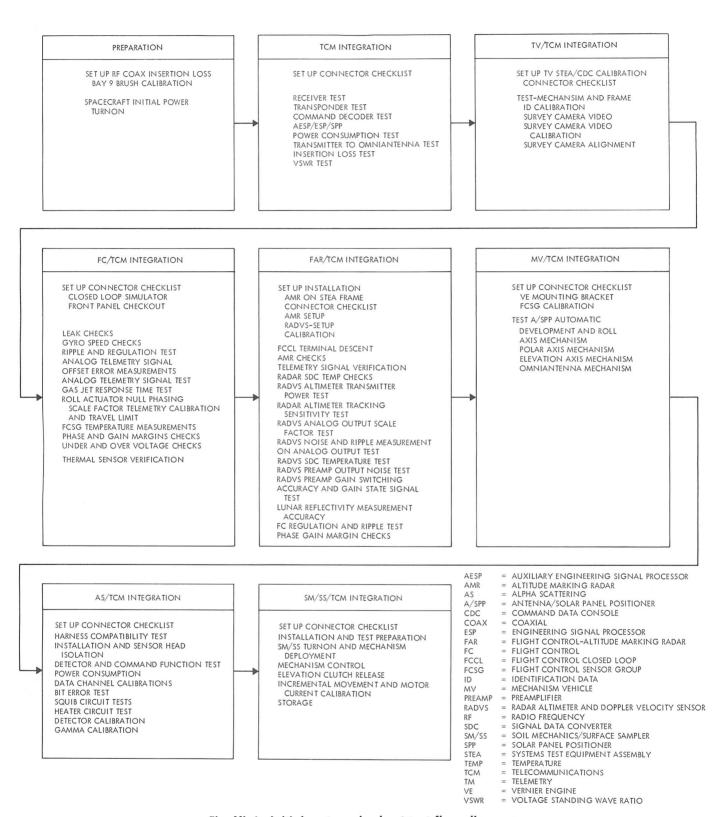
Fig. XI-6. Initial system checkout test flow diagram
