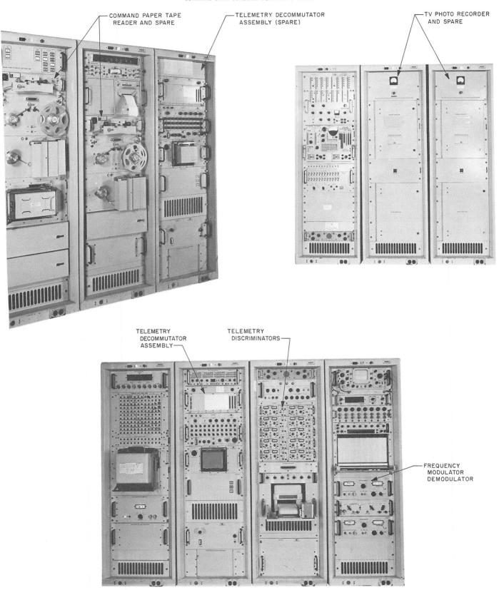
Fig. VII-4. The CDC equipment for DSIF
