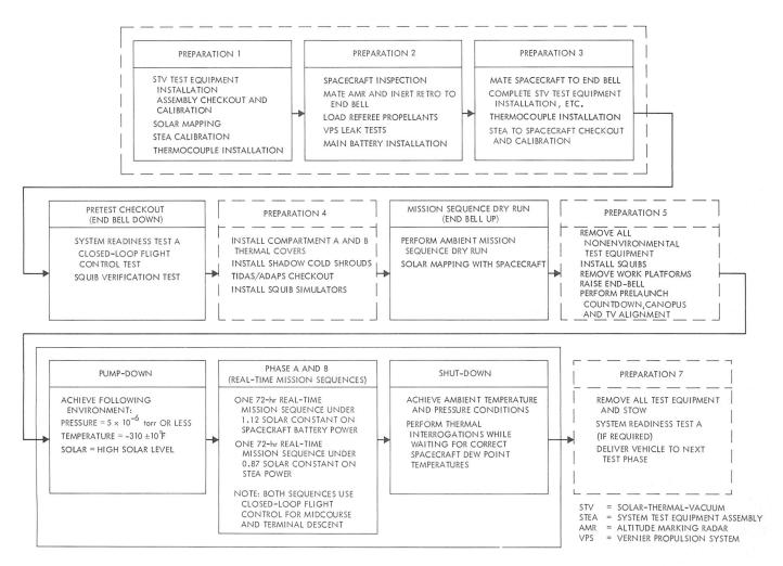
Fig. XI-10. Solar-thermal-vacuum test phase flow diagram
