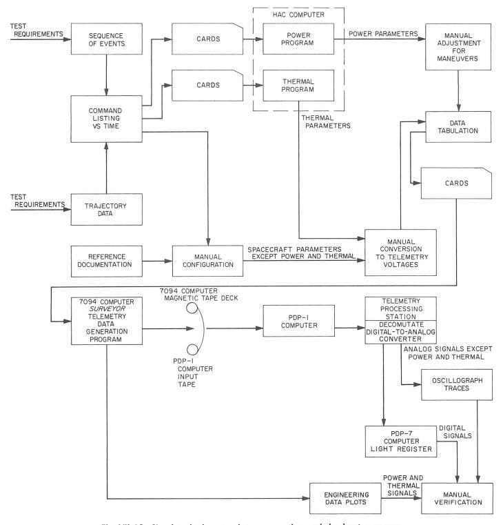
Fig. VII-12. Simulated telemetry data preparation and checkout sequence
