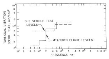
Fig. X-16. Comparison of the 95% flight equivalent torsional sinusoidal vibration environment and the specified torsional sinusoidal vibration environment for the S-9 structural test vehicle
