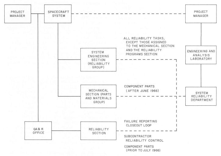
Fig. XII-5. Surveyor reliability task assignments and interface
