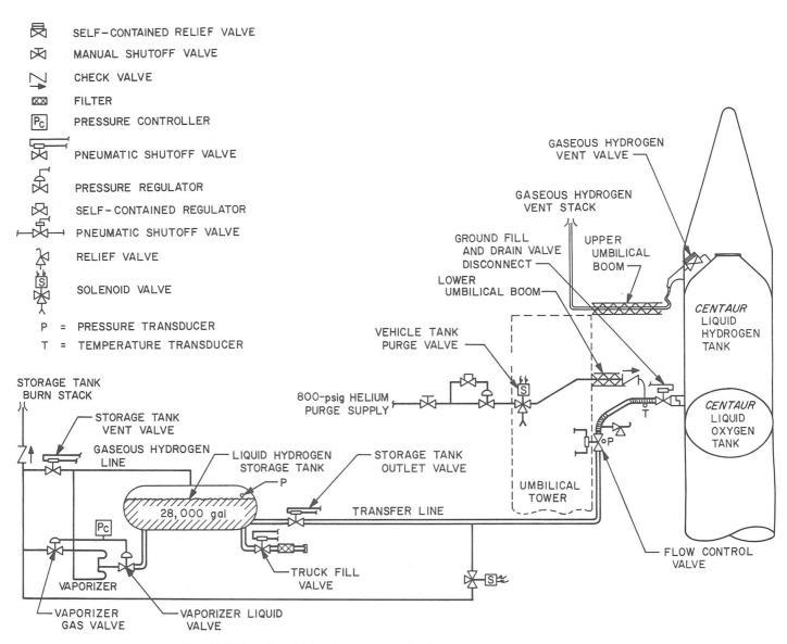
Fig. VIII-26. Liquid hydrogen transfer system, Launch Complex 36
