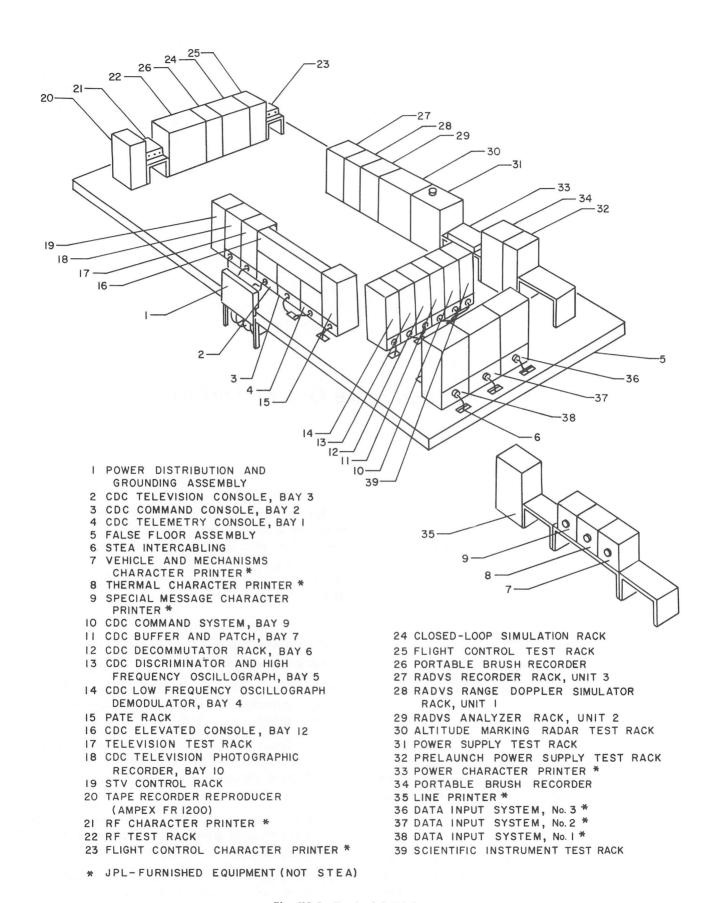
Fig. IX-1. Typical STEA layout
