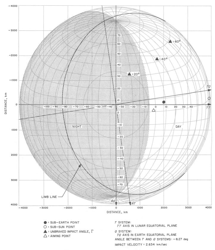
Fig. VI-20. Moon in B-space for typical trajectory
