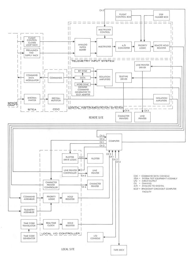
Fig. XI-3. Spacecraft checkout functional block diagram
