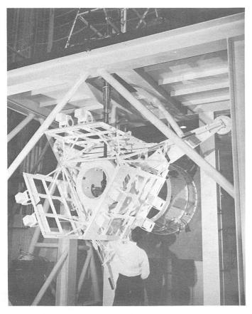
Fig. VIII-18. Spacecraft separation system test configuration
