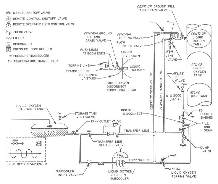
Fig. VIII-27. Liquid oxygen transfer system, Launch Complex 36B
