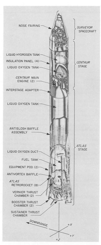
Fig. VIII-2. Atlas (SLV-3C)/Centaur/Surveyor space vehicle configuration
