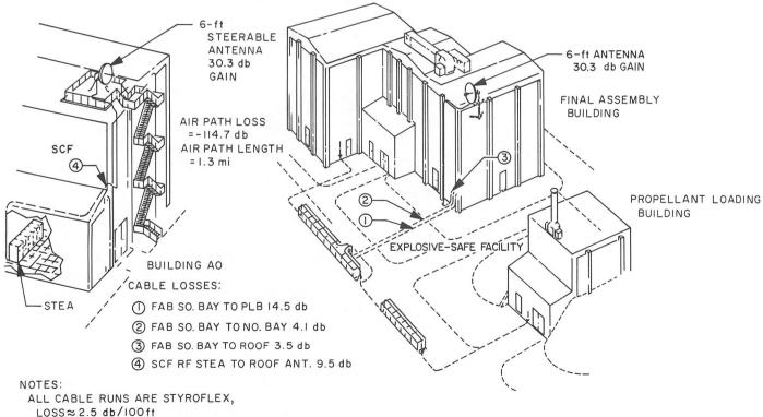
ALL CABLE RUNS ARE STYROFLEX, LOSS≈ 2.5 db/100ft STYROFLEX CABLE RUNS ARE PRESSURIZED WITH DRY NITROGEN
