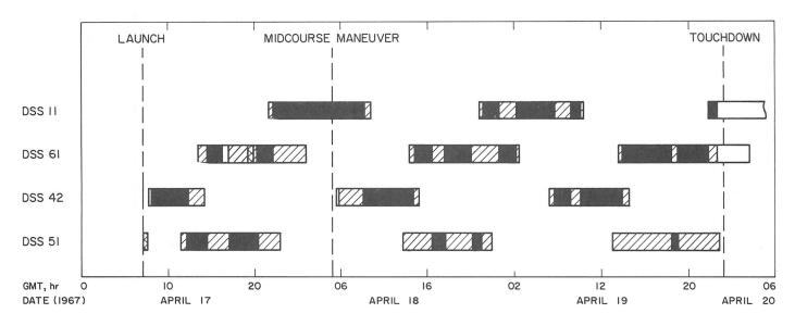
ONE-WAY DOPPLER ☐ THREE-WAY (NONCOHERENT) DOPPLER ☐ TWO-WAY DOPPLER ☐ VISIBLE: NO USABLE DATA
