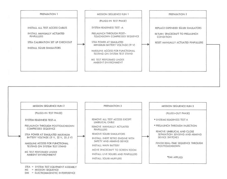
Fig. XI-8. Mission sequence/electromagnetic interference test phase flow diagram
