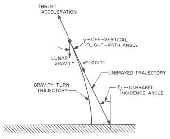
Fig. VI-9. Gravity turn descent geometry
