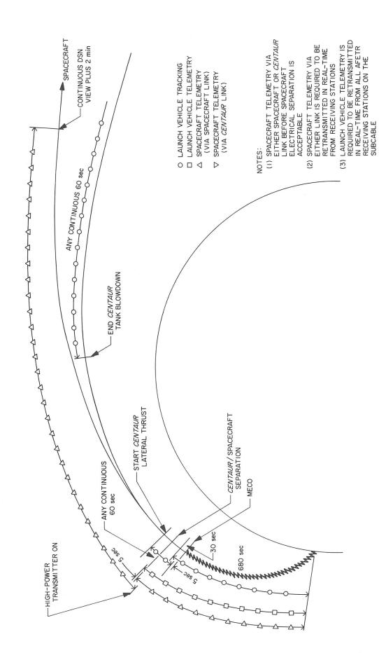
Fig. VI-31. Near-earth class I T&DS requirements for direct-ascent launches
