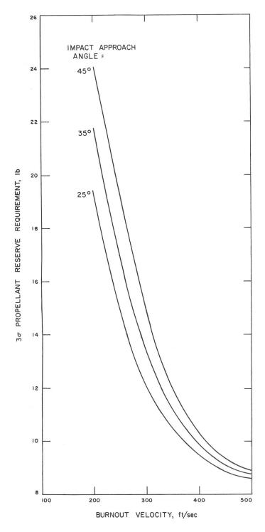
Fig. VI-22. Vernier propellant reserve
