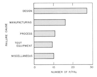
Fig. XII-22. Surveyor vernier engine problem/failure reports by failure cause
