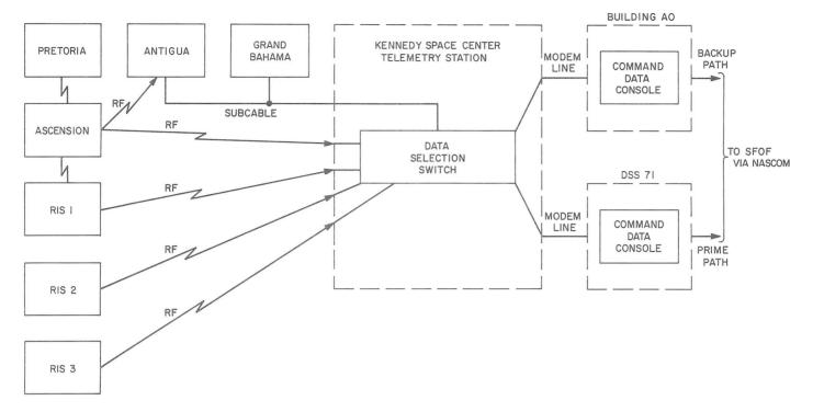
Fig. VII-21. Surveyor real-time spacecraft telemetry data transmission system
