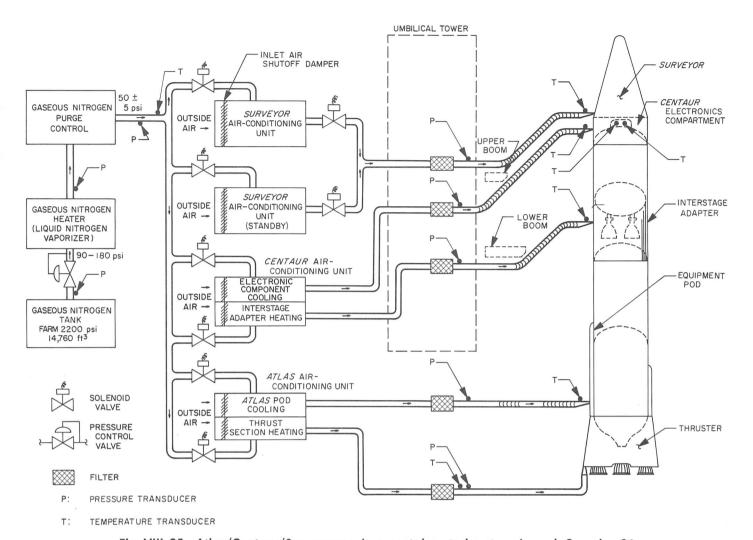
Fig. VIII-25. Atlas/Centaur/Surveyor environmental control system, Launch Complex 36
