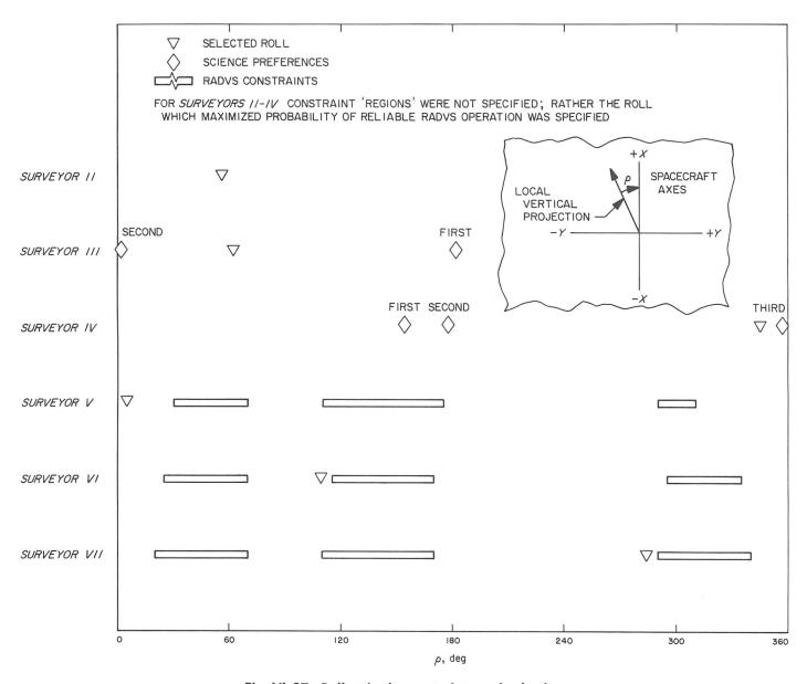
Fig. VI-27. Roll attitude constraints and selections
