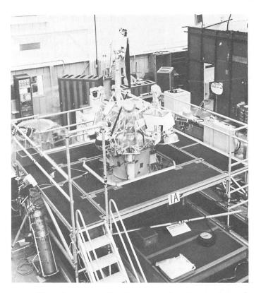
Fig. IX-6. Setup for vibration tests showing workstand
