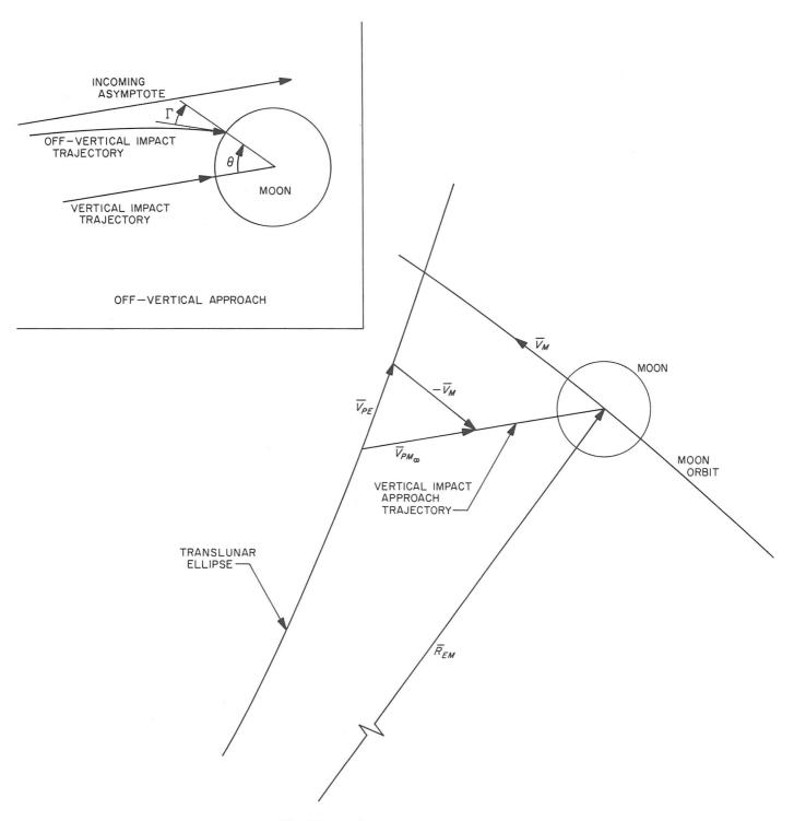
Fig. VI-4. Lunar encounter geometry
