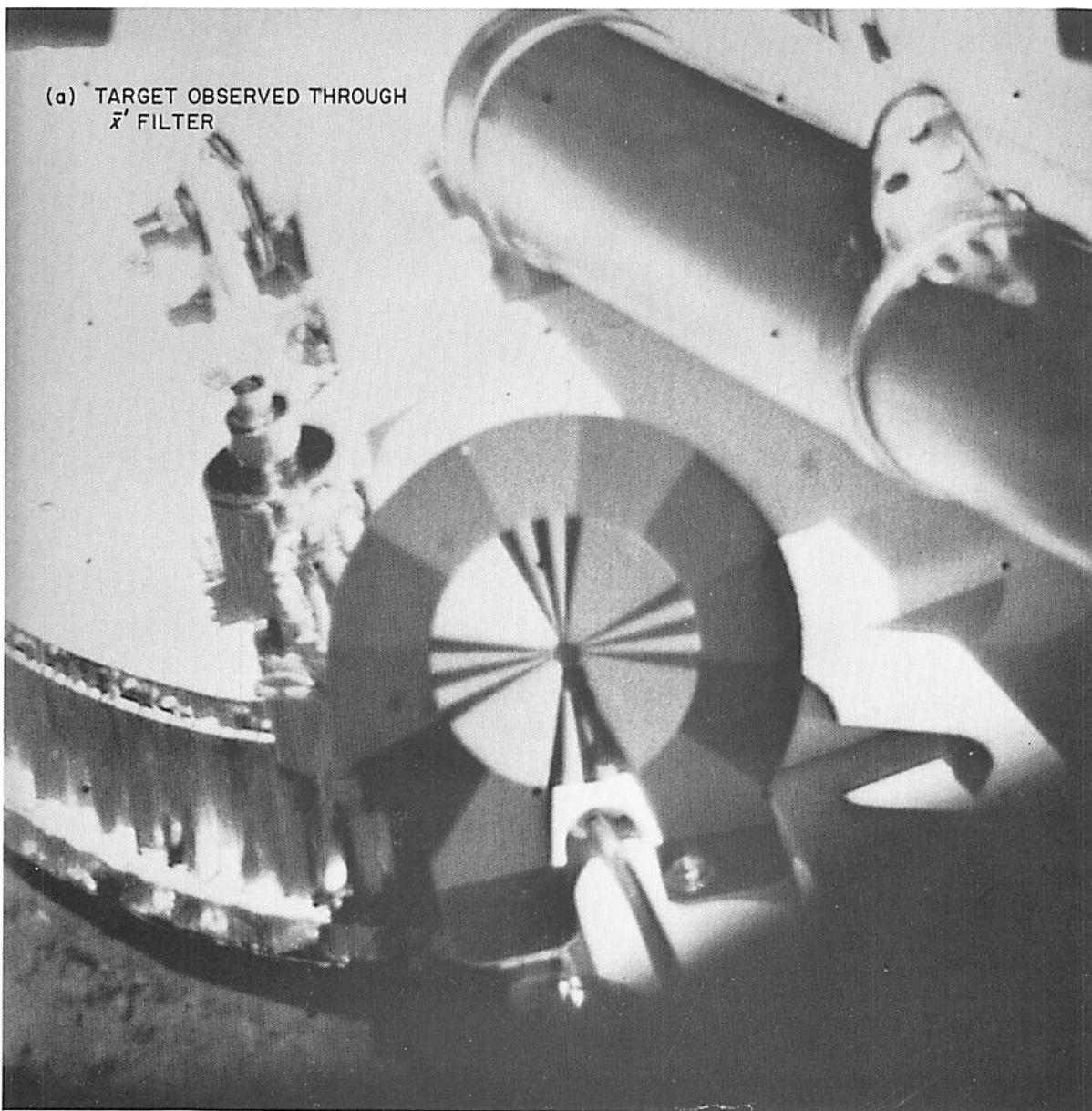
Fig. III-5. Photometric target on footpad 2
