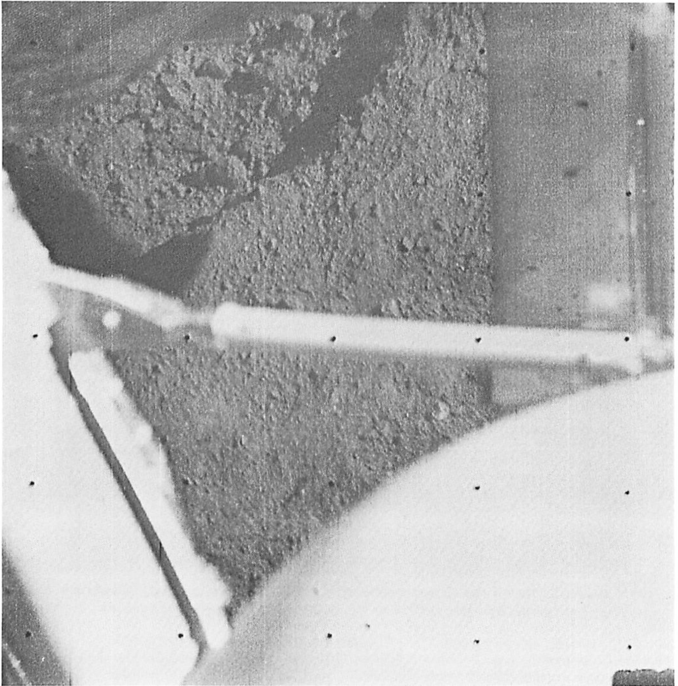
Fig. VI-12. Computer-processed picture of surface depression made by crushable block assembly 3. (Note depression made in upper left-hand corner; part of a propellant tank obscures the imprint in extreme left-hand corner. Sun angle is 41^\circ and from the right of the picture.)
