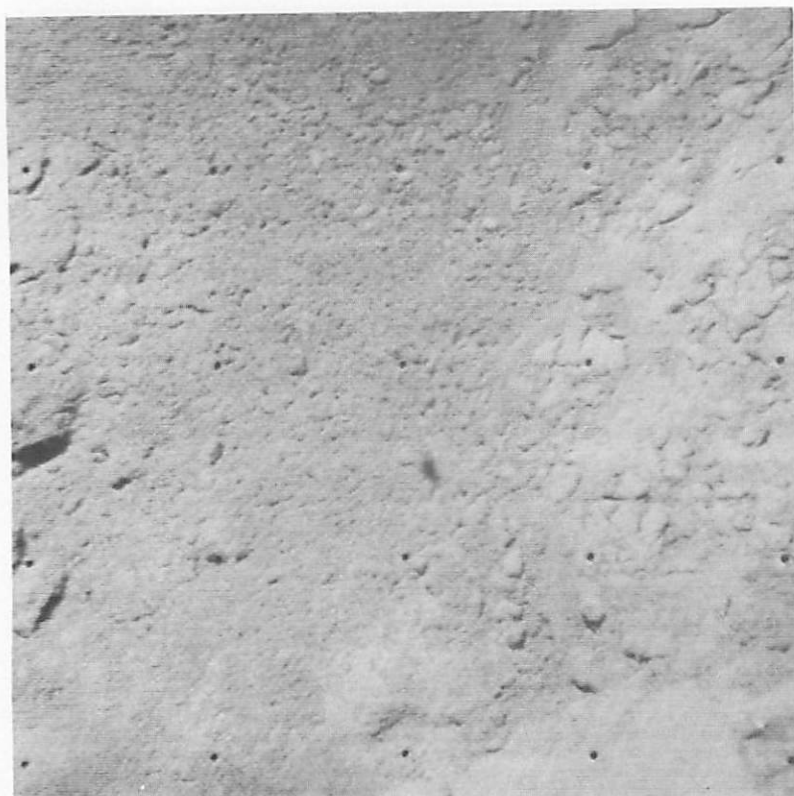
FIGURE 4-42. — Soil disturbed by vernier engine 1 firing. Soil fragments seen in area L probably have been moved along the surface without being overturned because their tops are formed of light-colored surface soil (day 321, 11:47:26 GMT).
