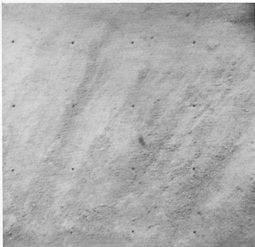
FIGURE 4-43. — Rays of dark fine soil ejected by vernier engine 1 during hop (day 321, 11:32:52 GMT).
