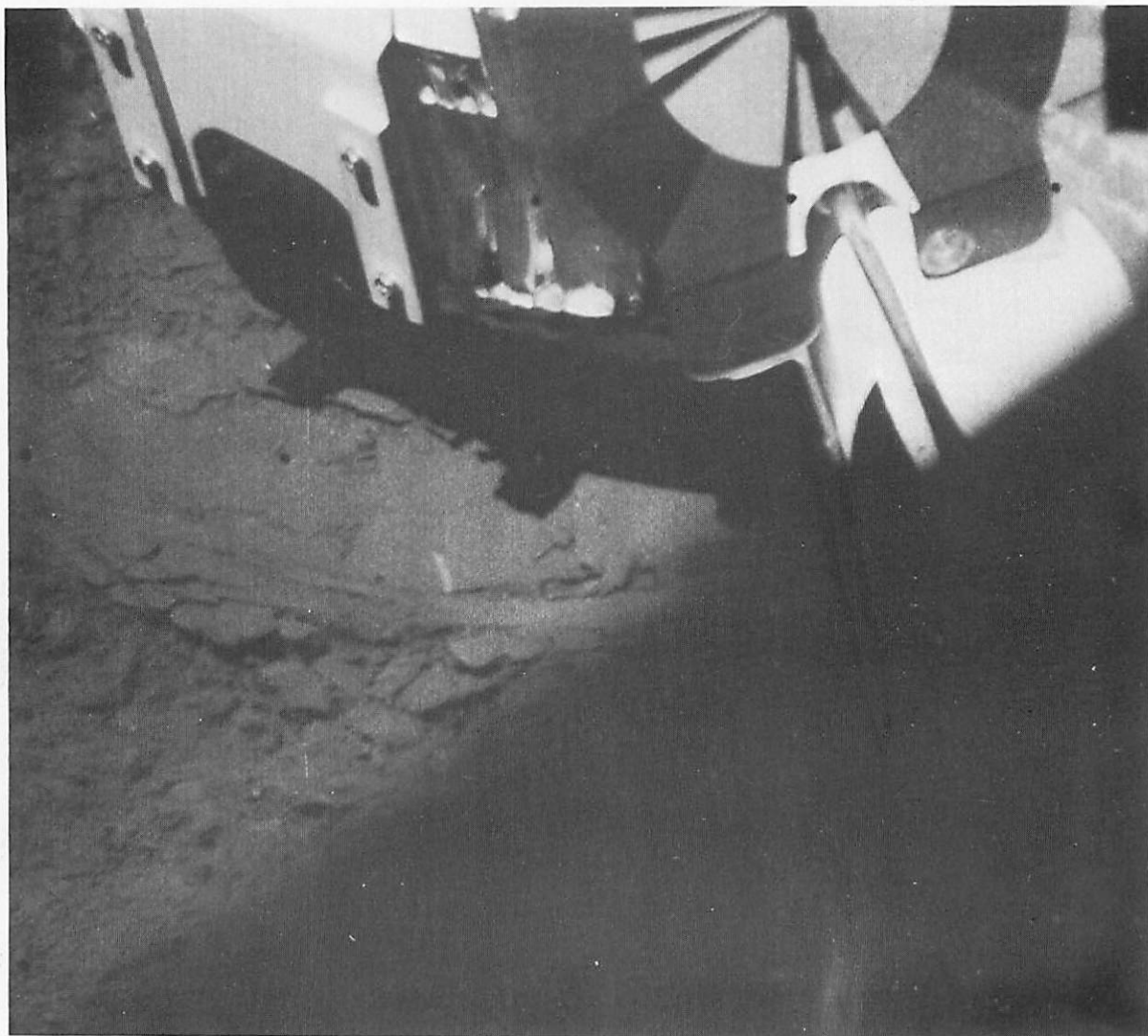
FIGURE 4-11. — Compressed lunar soil in the bottom of the footpad 2 imprint made during the initial landing (day 320, 03:35:09 GMT).
