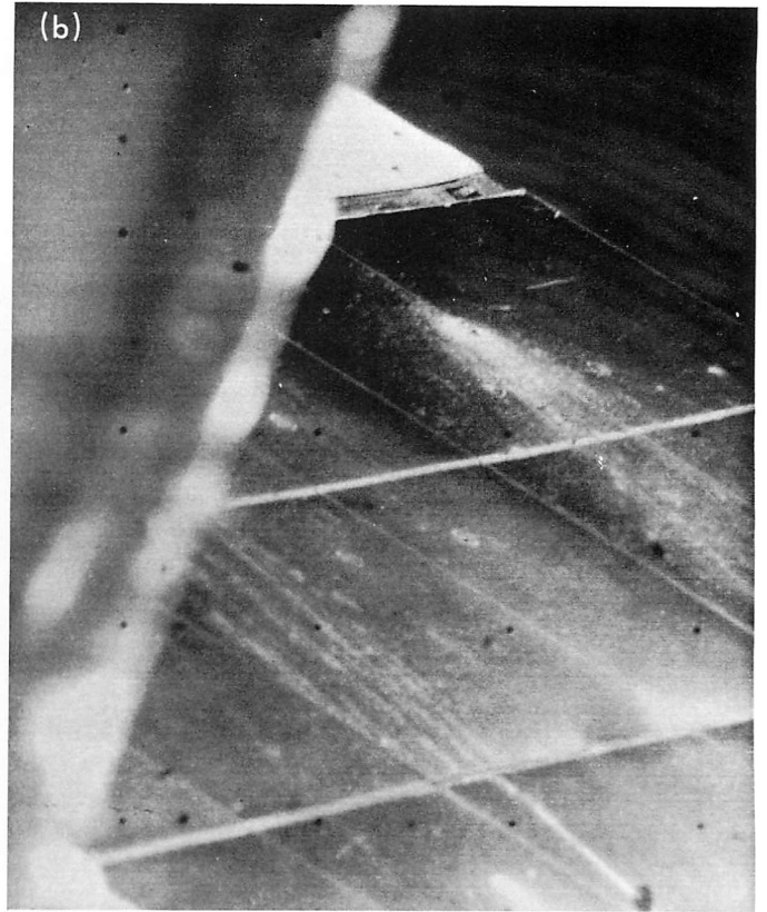
Fig. IV-39. Top of compartment B taken before and after the firing. A lump of material was transported to the compartment top and splattered in a direction away from vernier engine 1. (a) Day 255, 02:29:29 GMT. (b) Day 265, 05:48:58 GMT.
