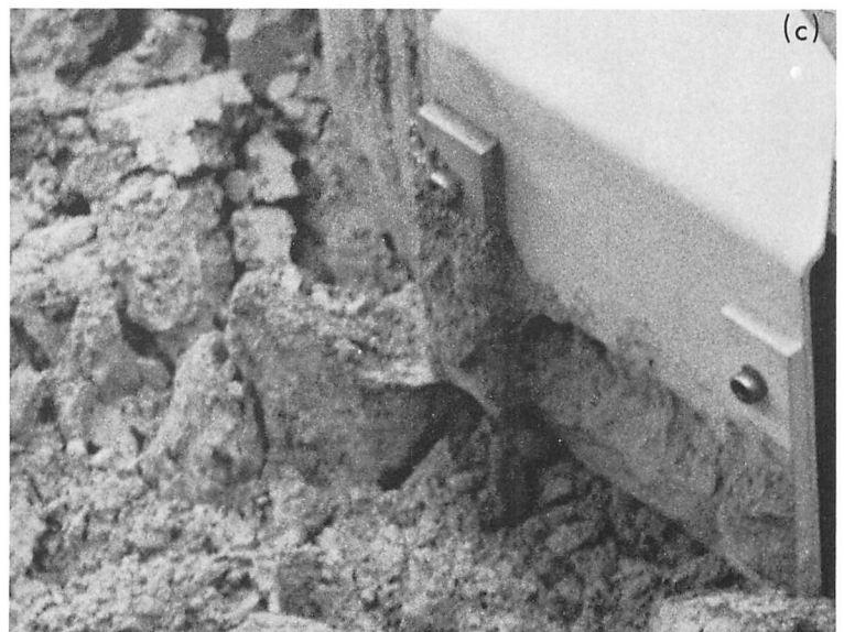
Fig. VIII-19. (a) Laboratory simulation of footpad 2 landing mode in 37–50 \mu Little Lake basalt. Velocity, depth of penetration, and distance were simulated. (b) Picture taken by Surveyor V of the side of trench dug by footpad 2. Note similarity to Fig. VIII-18a and VIII-18c (Day 258, 04:02:17). (c) Closeup of footpad and magnet assembly used in laboratory simulation studies of landing (Fig. VIII-18a). Six such landings were performed; all results were similar. Note material on control bar on the right, material in the honeycomb and clumped on the magnet, covering the attachment screws. The increased humidity in the laboratory may have caused results similar to the apparent vacuum cohesion on the moon.
