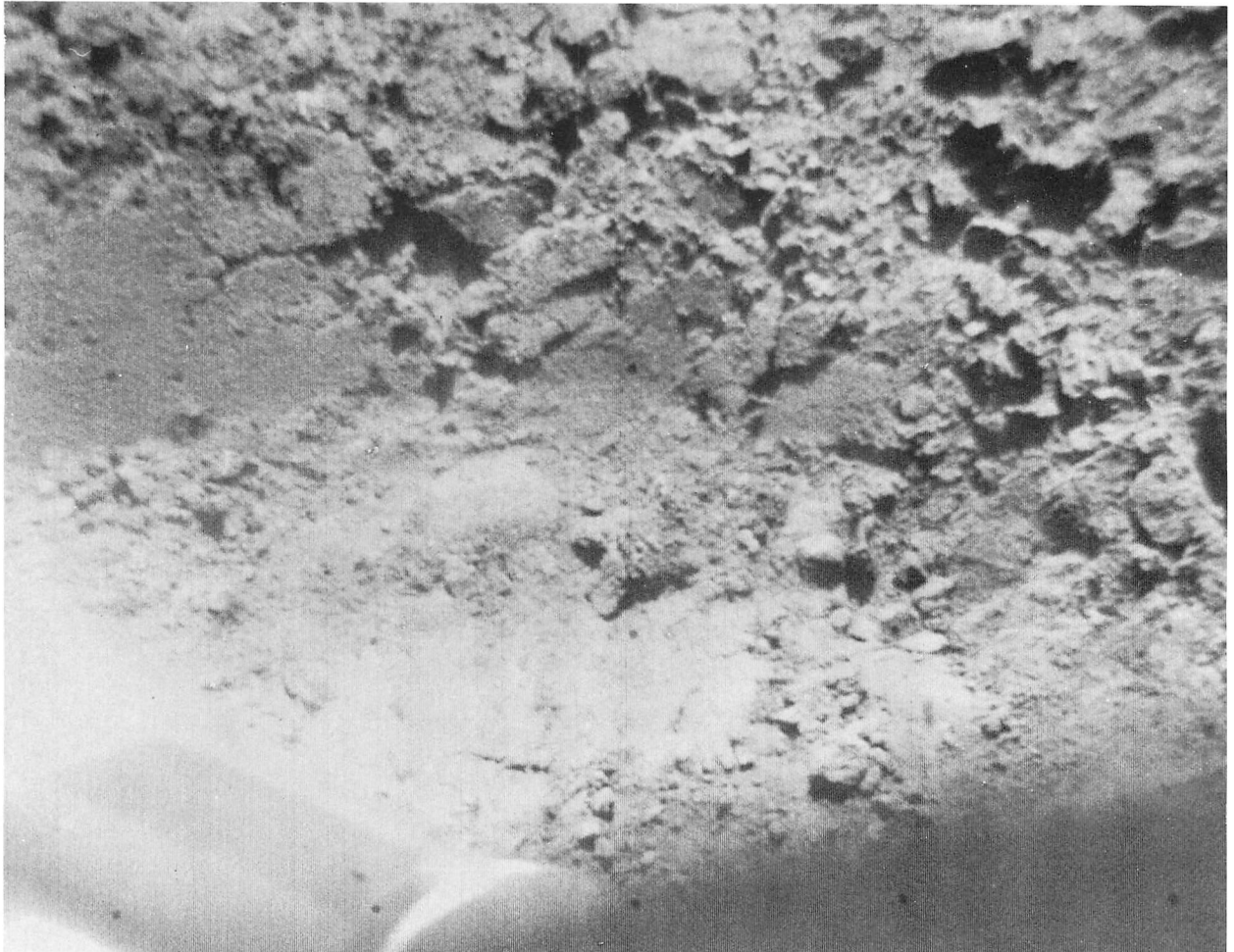
Fig. IV-6. Narrow-angle picture showing detailed view of a part of the trench wall formed by the scraping action of footpad 2 (Day 257, 04:42:06 GMT).
