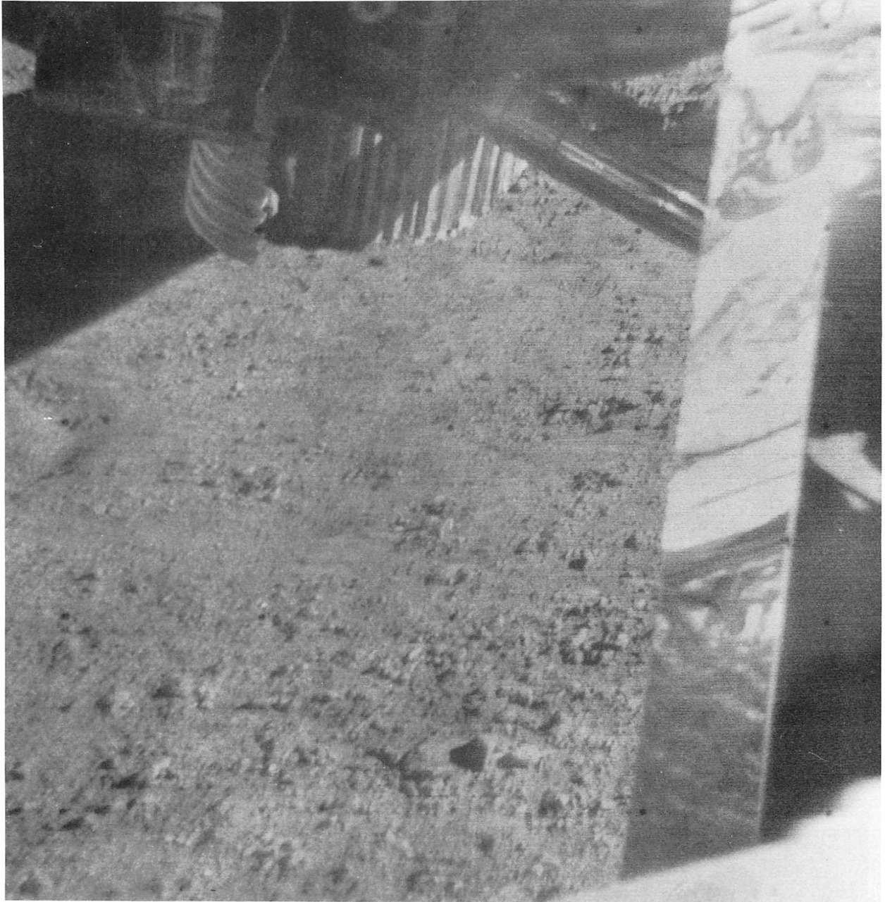
Fig. IV-14. Narrow-angle view taken through the auxiliary mirrors showing the bottom of crushable block 3. A small rock or clod, seen wedged between the block and the thermal shield, was probably picked up during the first landing impact (Day 263, 11:47:23 GMT).
