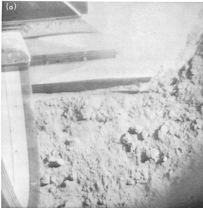
Fig. IV-31. Gold-plated face D (see Figs. IV-27 and IV-28) of the sensor head. (a) Pre-firing picture; face D is highly reflective (Day 255, 05:06:27 GMT). (b) Post-firing picture; face D is nonreflective (Day 257, 07:15:09 GMT).
