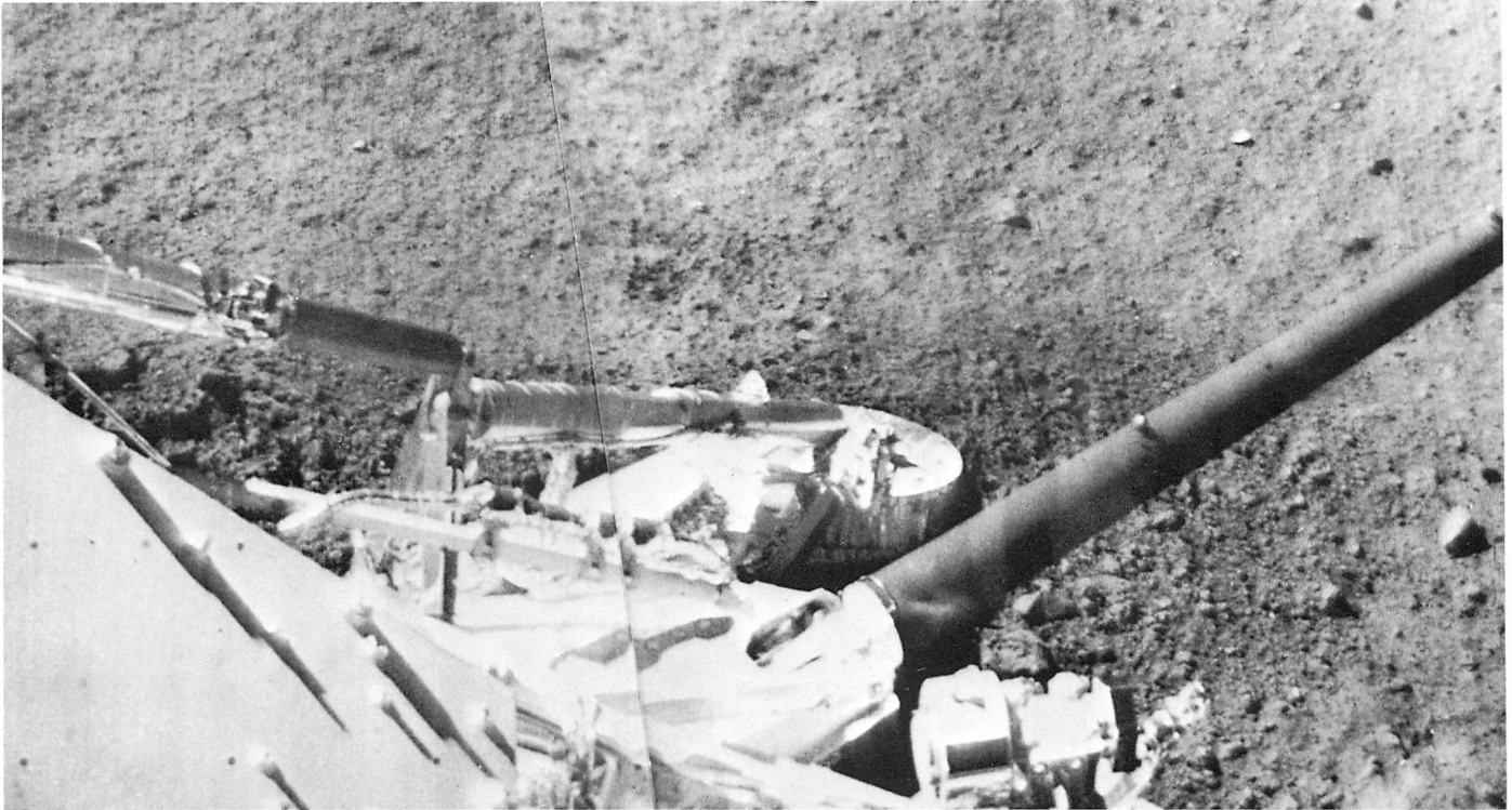
Fig. IV-9. Wide-angle mosaic of spacecraft landing leg 3 and footpad 3. A portion of the trench formed by footpad 3 during the landing can be seen through the leg structure. The throwout pattern of lunar material ejected during the landing is visible above and to the right of the footpad (Day 263, about 06:50 GMT; Catalog 5-MP-33).
