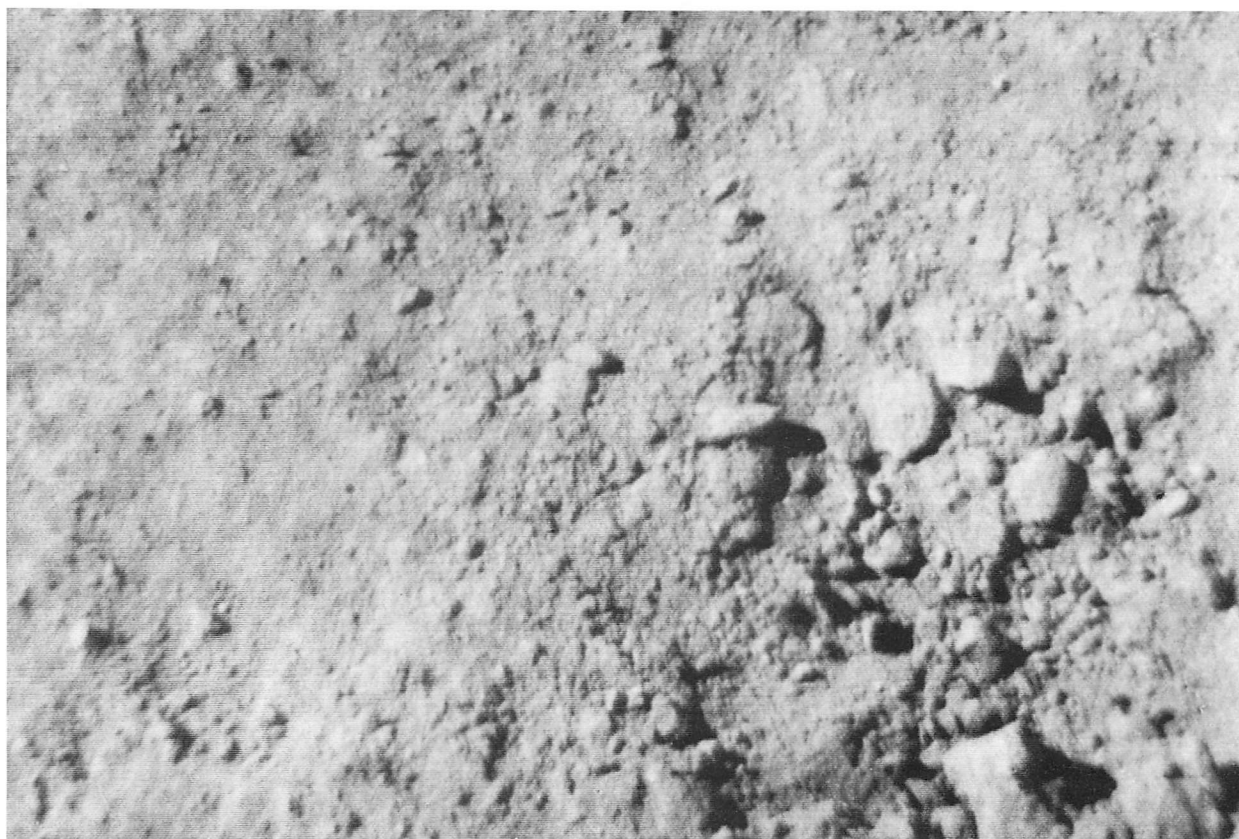
Fig. III-20. Narrow-angle picture showing fragments in small crater on the north wall of the Surveyor V crater. The small crater is lined with fragments similar to those exposed in the trench dug by footpad 2 during landing. Most of the fragments are aggregates of fine particles; complex aggregates and individual, bright, rocky chips also appear to be present (Day 264, 12:12:24 GMT).
