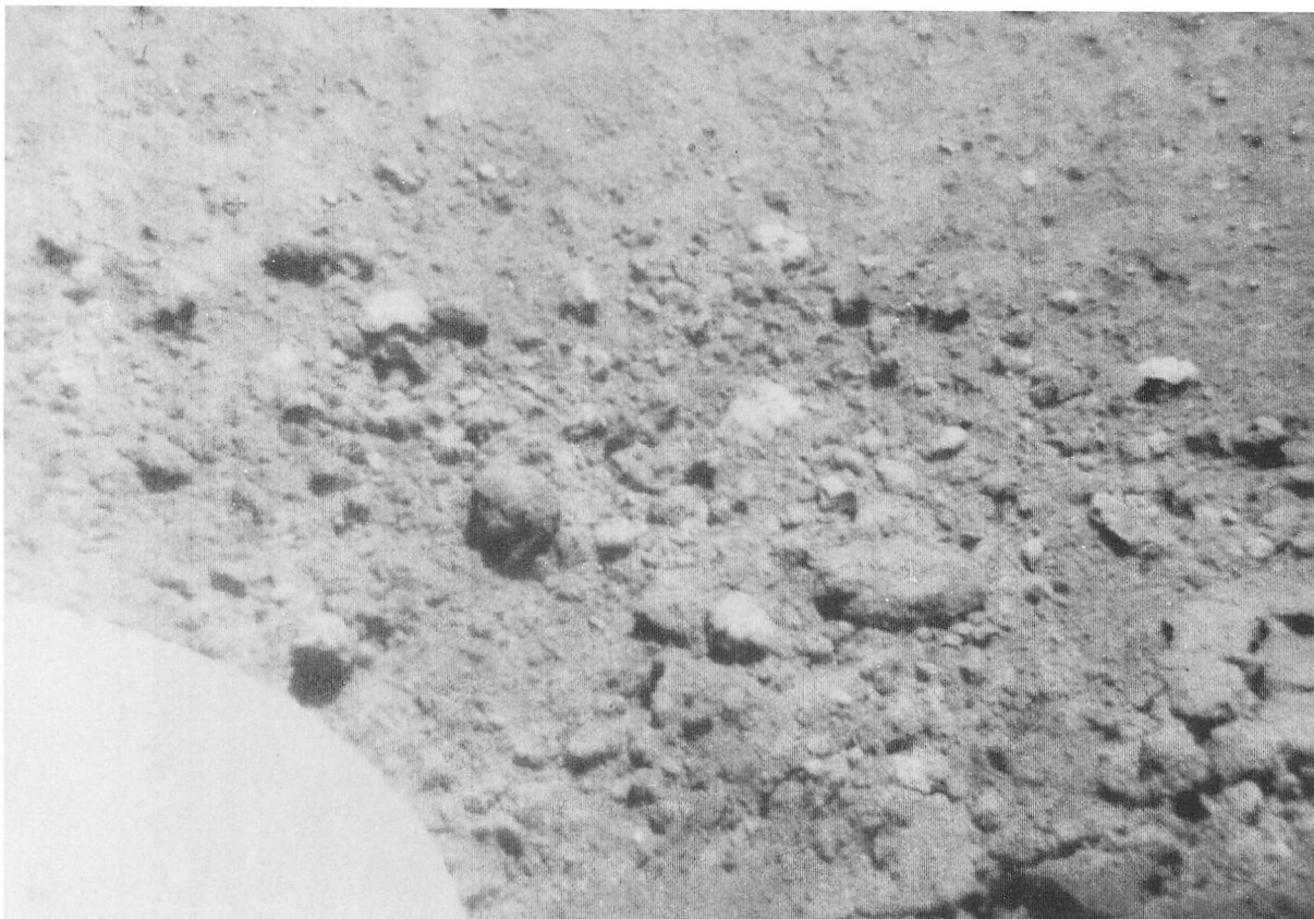
Fig. III-18. Area V-A: an area used to determine size-frequency distribution of fragmental material thrown onto the lunar surface in front of footpad 2 during landing. Most of the fragments are aggregates of fine particles. The bright fragments probably are pieces of coherent rock. Some dark, lumpy objects may be aggregates of aggregates. Smallest fragments resolved in this picture are about 1 mm across, and the largest fragments are about 3 cm across (Day 258, 08:40:04 GMT).
