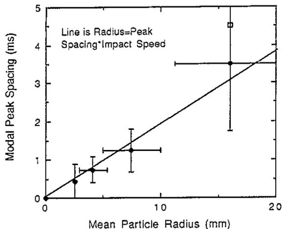
**Figure 11.** Correlation of peak spacing with particle size. A moving average is subtracted from the impact signature, and the spacings between positive-going crossings of the  $3\sigma$  levels are placed into bins 0.5 m s wide. The location of the most popular (modal) bin is plotted again particle size.
