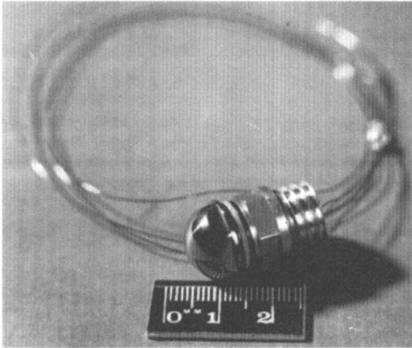
Figure 2. A photograph of the penetrometer sensor head.
