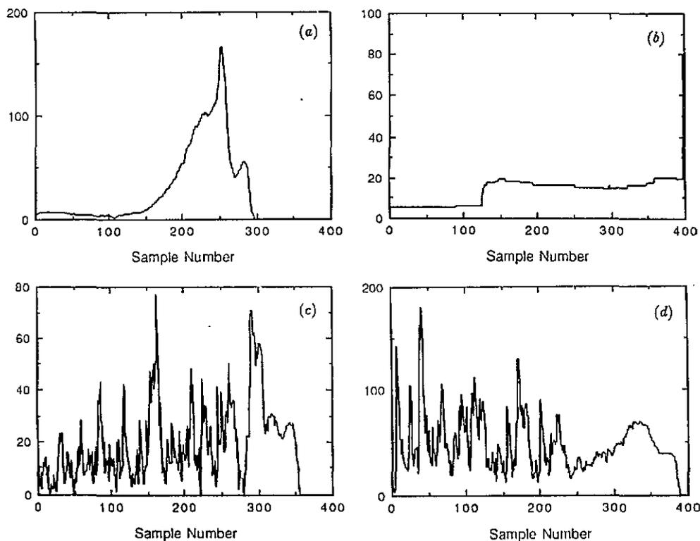
**Figure 10.** Sensor output (after pseudo-log amplification; units are arbitrary) for transducer drops at  $5 \text{ m s}^{-1}$  into various materials. Samples are at  $10 \text{ kHz}$ , so sample number 200 corresponds to  $20 \text{ m s}$ , or  $10 \text{ cm}$  depth. Materials are (a) sand, (b) clay, (c) fine gravel (particle size about  $8 \text{ mm}$ ) and (d) medium grade gravel (particle size about  $15 \text{ mm}$ ).
