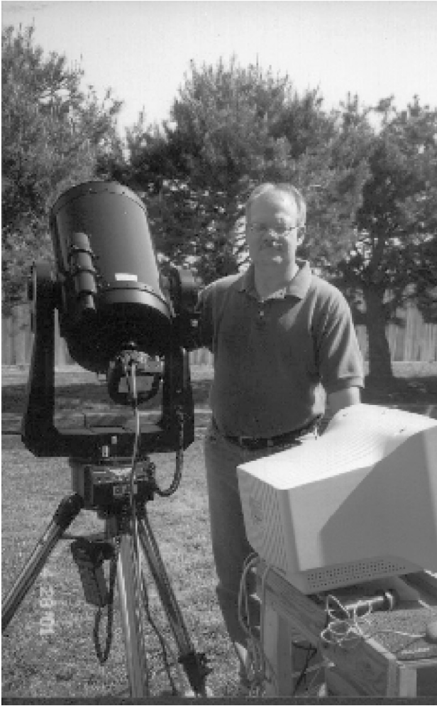
Fig. 2. Author Doug West with observing equipment. Modern computer-guided telescopes can be set up within a few minutes, making a permanent observatory installation largely unnecessary. For monitoring projects the small manpower overhead in setup outweighs the larger aperture of mountaintop observatories.
