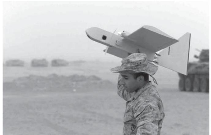
**Fig. 1 A Dragon Eye UAV about to be hand-launched during Operation Enduring Freedom in Kuwait in 2003. This vehicle is twice as massive as the concept discussed in this paper.**
