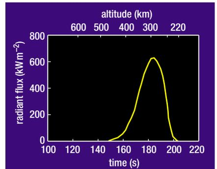
6: The emission from the shock layer on to the front shield for the Huygens probe peaks at some  $600 \text{ kW m}^{-2}$ , or around 500 times the solar constant. The emission pulse lasts 20–30 s, during which the probe traverses the altitude range 400–250 km, above most of the atmospheric haze.
