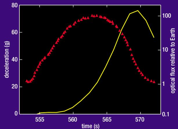
4: The CN line emission and its evolution with time is sensitive to the abundance of carbon atoms in the atmosphere. These data (triangles), recorded by the PAET radiometer, are fitted by a model (curves – see Whiting *et al.* 1973) with best fit corresponding to the known carbon dioxide abundance (~300 ppm). In this regime, emission has a nearly linear dependence on carbon abundance – this linearity will not extend to the very high levels of carbon in Titan's methane-rich atmosphere.
