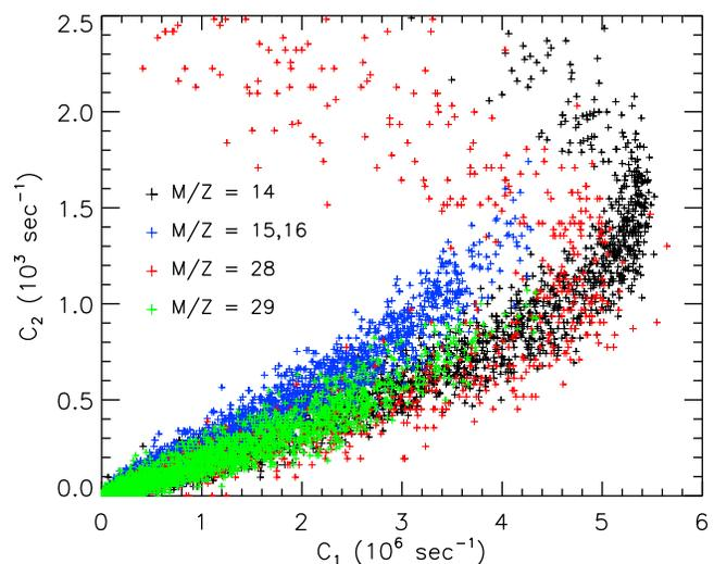
**Figure 4.** The C2 count rates as a function of the C1 count rates, for channels 14, 15, 16, 28 and 29. The data points from all flybys in our sample have been included. The C1–C2 relations indicate that the saturation characteristics are species dependent.
