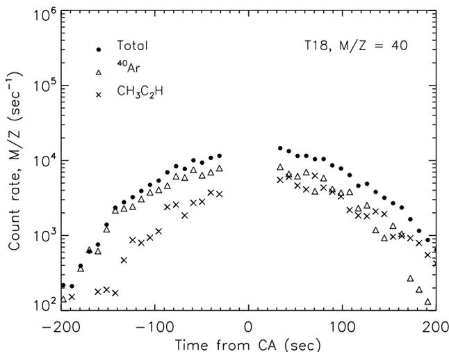
**Figure 2.** The count rate in mass channel 40 as a function of time from CA for the T18 flyby. Different symbols stand for the total count rates, the count rates contributed by <sup>40</sup>Ar and CH<sub>3</sub>C<sub>2</sub>H, respectively. The relative contributions of different species are calculated with the nominal algorithm (see text for details). The apparent asymmetry in CH<sub>3</sub>C<sub>2</sub>H is an indication of the wall chemistry effect.
